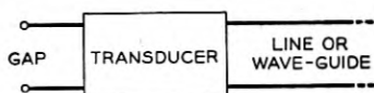
Fig. 117.—A 4-terminal transducer is the most general connection between the oscillator gap and a line or wave guide.
