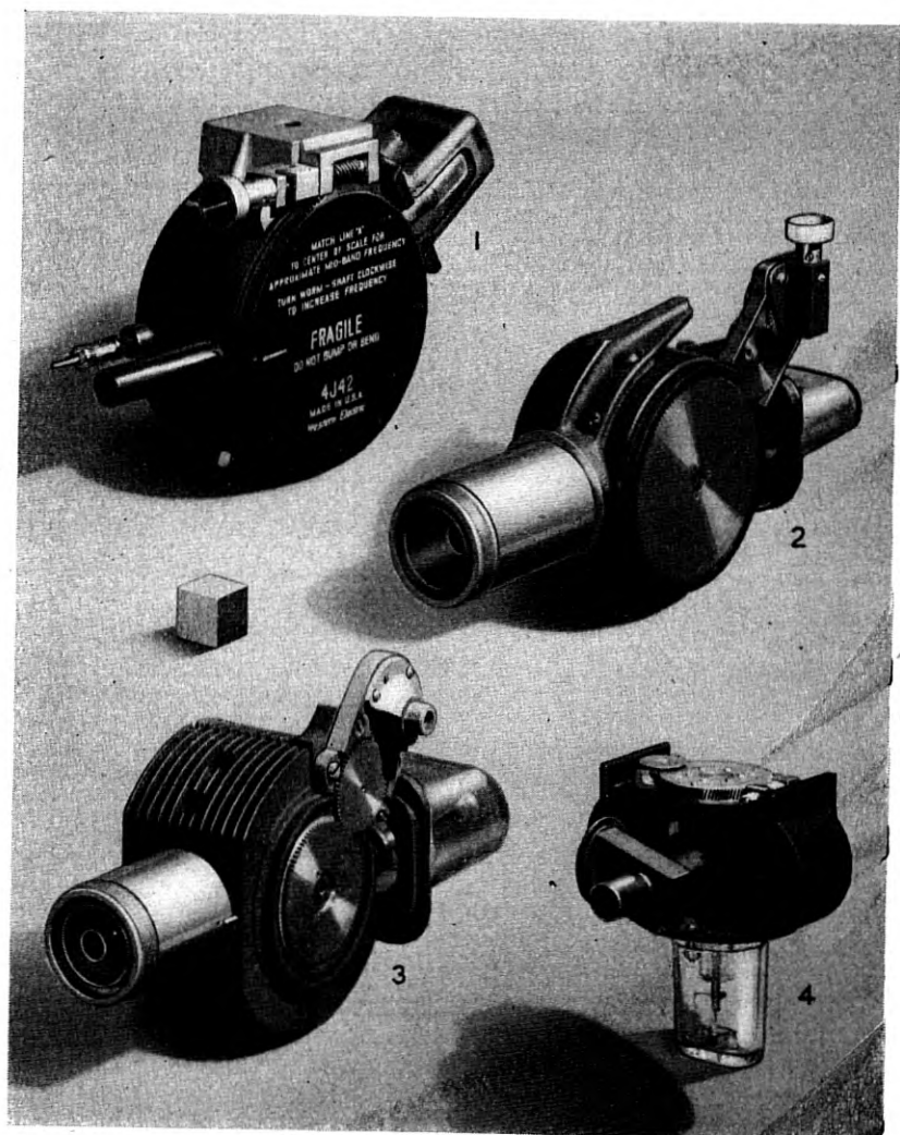
Fig. 43—Four tunable magnetron oscillators. They are: (1) the 4J42 magnetron (40 kw., 660 to 730 mc/s); (2) the 4J51 magnetron (275 kw., 900 to 970 mc/s); (3) the 5J26 magnetron (600 kw., 1220 to 1350 mc/s); and the 2J51 magnetron (55 kw., 8500 to 9600 mc/s).
