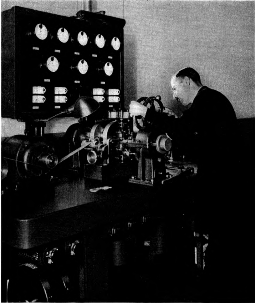
Fig. 6—Twenty roll cold-reduction mill for producing thin sheet materials for experimental studies.
