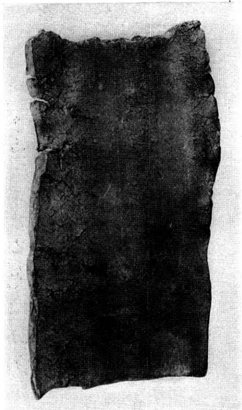
Fig. 2—View of piece of old cable sheath made of commercially pure lead, which failed in service from intercrystalline fracture.
