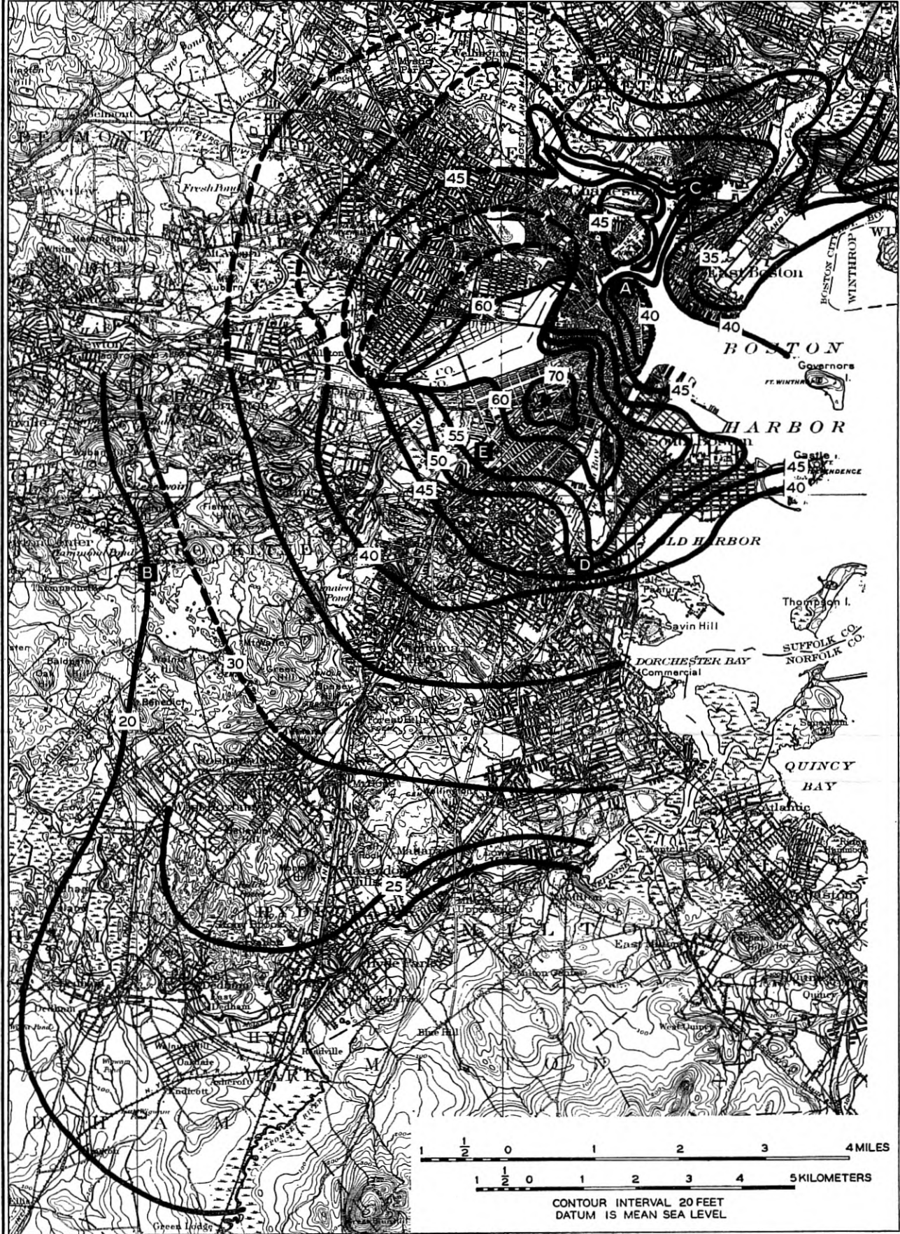
Fig. 8—Field strength contour map of Boston, Mass. Transmitter located at Berkeley and Stuart Streets as shown by the solid circle. Frequency = 34.6 mc. Field strength in decibels above one microvolt per meter with one ampere in a half wave antenna.
