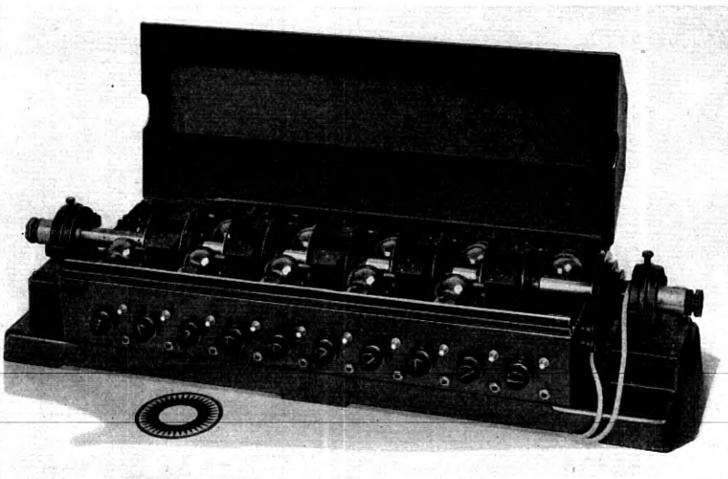
Fig. 23—Ten disk optical tone generator.
