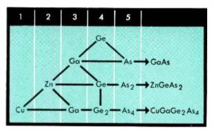
Method of combining elements to form semiconductors with 4:1 valence electron-to-atom ratio.
