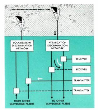
The effect of mutual coupling between the transmitting and the receiving antennas on the same tower. Extra IF filter helps reduce coupling loss due to interference between the two antennas.
