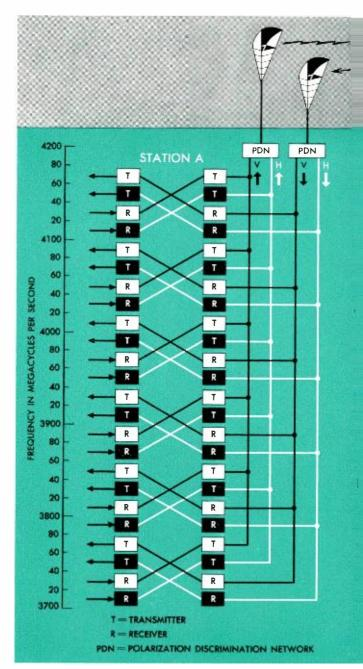
TD-2 system with interstitial channels. The use of entire broadband channel between 37 and 42 kmc
