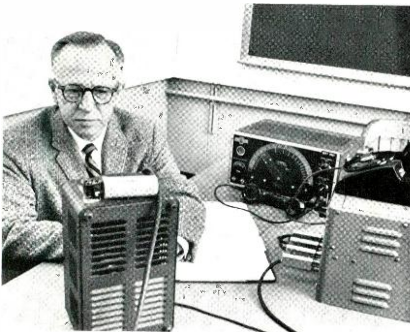
F. L. Crutchfield with special testing arrangements used in Crystal Lake trial. Mr. Crutchfield reads meter on control panel. Other components of the equipment are the sweep oscillator, rear; and the transmission measuring set, right.
