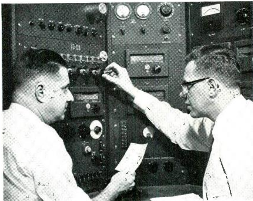
The author (right) and R. C. Gee check the performance of high-purity nickel cathodes as revealed in life tests of tubes.
