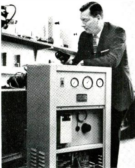
Author J. M. Jackson checks pressure for refrigeration dryer designed for small central offices.
