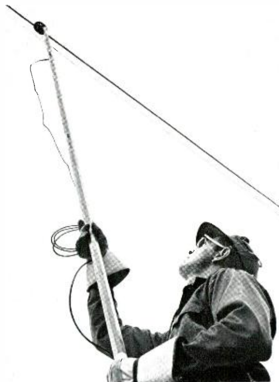
The 105 test set. J. D. Appar moves test set along a cable to locate faults in cable-conductor.
