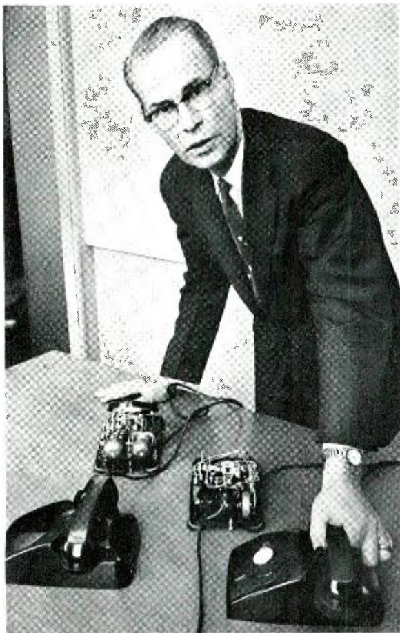
Author shown with the tone-ringer telephone and a standard 500 set. Both casings have been removed to show difference in circuit components.
