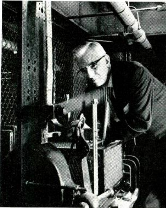
E. L. Alford observes climber, center, with strap coming from footrest, being fatigue-tested. Slight blur, center, is moving arm, which cycle-stresses adjustable climber to simulate use in the field.
