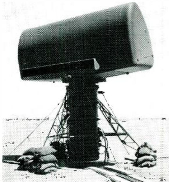
Acquisition radar constantly surveys the area to be defended in case of attack. This equipment identifies potential enemy targets at long range.
