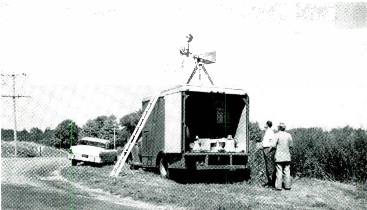
Mobile laboratory for measuring radar interference. J. M. MacMaster, of the Transmission Engineering Department, is adjusting the pickup horn
