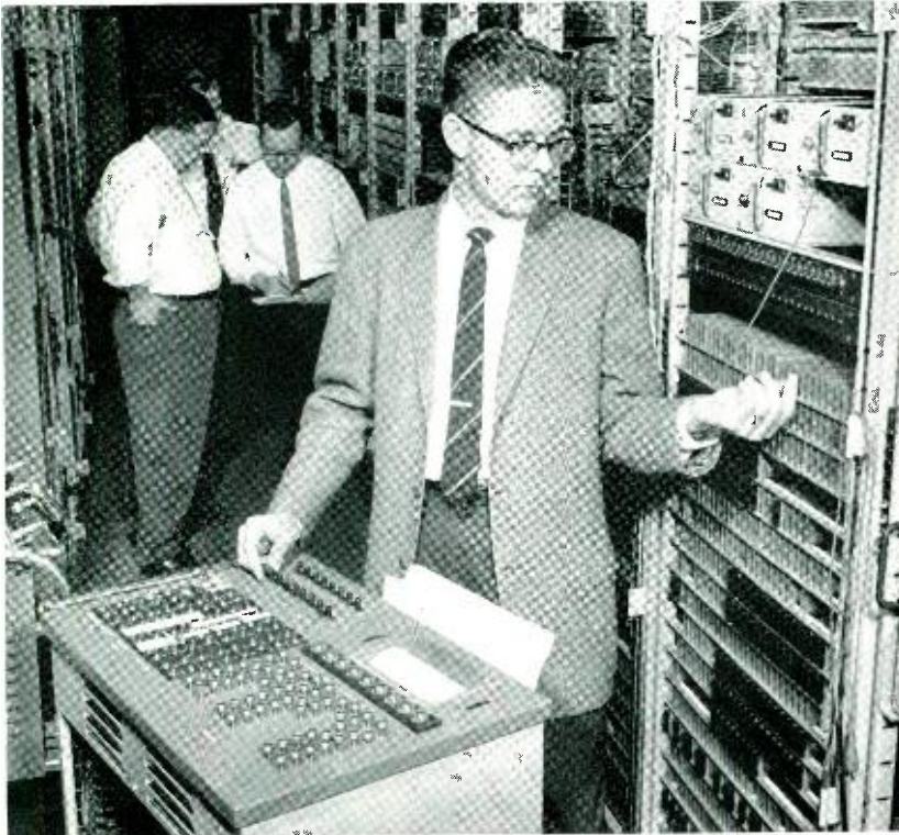
Author using central control manual tester. Equipment tests operation of central control logic circuits by putting control orders worked out elsewhere into the system.
