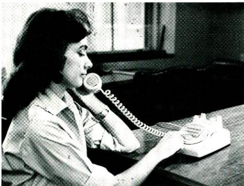
Mrs. Carole Rustako of the Laboratories demonstrates the first step in dialing SH-1, one of the office codes used in the Elgin trial. She is using an exploratory model similar to those used in the actual trials.
