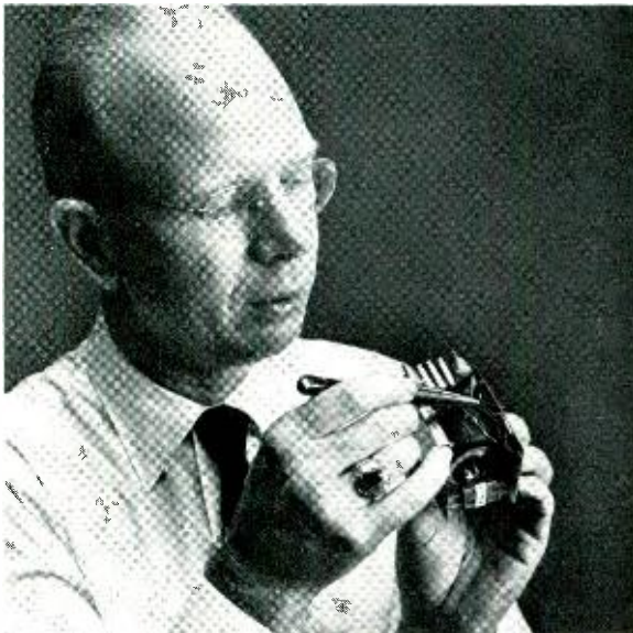
A computing amplifier before it is enclosed. Within this space, besides the magnetic cores and windings, are various precision resistors, adjusting potentiometers, and semi-conductor diodes.
