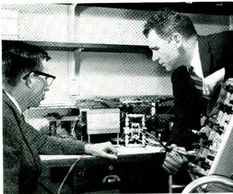
William W. Anderson, left, and Marion E. Hines inspect laboratory model of new traveling-wave solid-state amplifier. Device combines negative resistance of Esaki diodes and one-way attenuation of ferrite strip transmission line arrangement for improved amplification.
