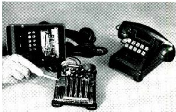
Telephones used in the 1948 trials of push-button calling. Pencil shows transducer that picks up tones from plucked reeds (fixed to the base behind the key levers). Note arrangement of buttons.
