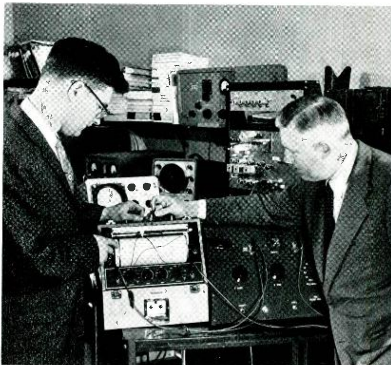
Robert L. Batdorf, left, and Donald E. Thomas inspect voltage-current curve of an Esaki diode just traced on new instrument. Measuring instruments such as this one must be constantly improved to keep up with the development of devices they measure.
