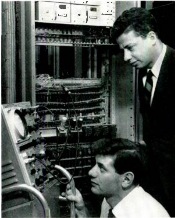
The author (right) with S. Bove test the scanner seen in the background; printed-wiring plug-in units can be seen in bottom part of the frame.
