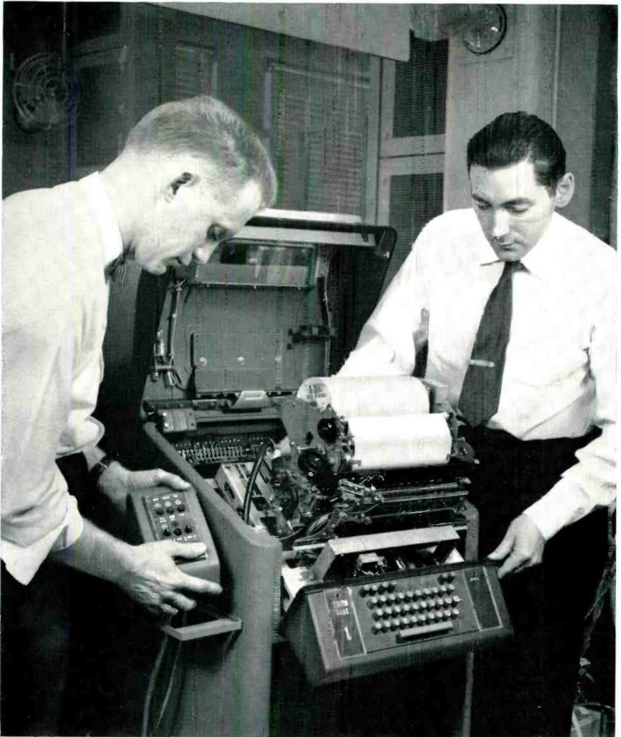
E. E. Barrett (left) placing key and lamp panel on a 28KSR station while L. M. Kolensky tips the typing unit forward to inspect the stunt box. New model teletypewriter unit has permitted improved systems that help solve the problems of "redundancy," "assurance" and "contention."
