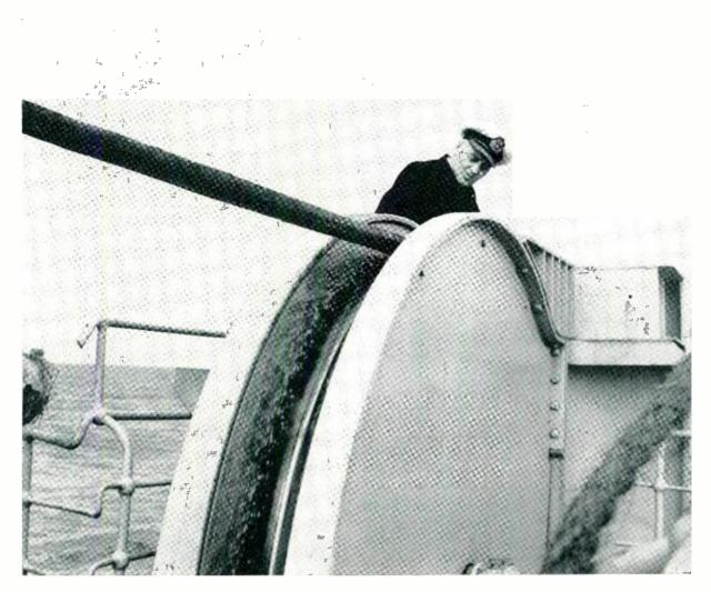
The transatlantic cable shown here paying out off the stern of the cable-laying ship H.M.S. Monarch. The fifty-one repeaters had to be
