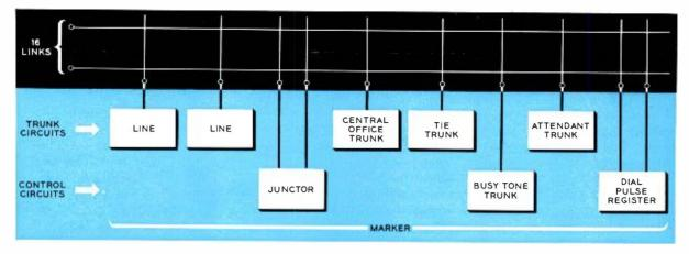
Diagram of linked crossbar switches showing approximate relationship of connecting and control
