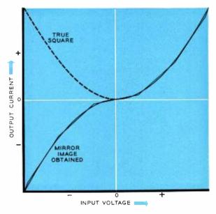
The square circuit input-output characteristics, showing the actual graph of straight-line approximations. Output current is approximately the square of input voltage, but minus is retained.
