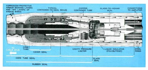
Internal construction of an undersea telephone cable repeater. Repeater enclosure is terminated at each end with a system of seals: glass-metal,
