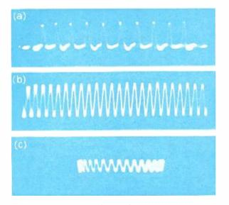
160 million pps timing pulses as seen on (a) broad-band tube, and (b) conventional tube. Part (c) represents a display of an 800 megacycle sine wave seen on the face of the broad-band tube.
