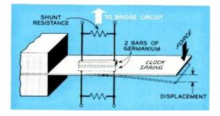
Displacement gauge constructed with crystals of germanium. Such gauges are up to two orders of magnitude more sensitive than common types.
