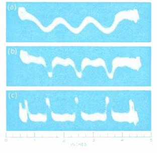
Photograph of the television monitor which shows the effects of the milli-microsecond timing pulses.
