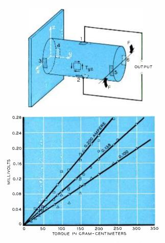
Configuration of the torsional transducer. Graph shows calibrations at different biasing currents.
