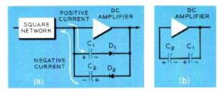
(a) Amplifier circuit to compute average square of its input voltage. Capacitors are connected in series with oppositely poled diodes  $D_1$  and  $D_2$ . (b) Circuit rearranged to "hold" the squared value.
