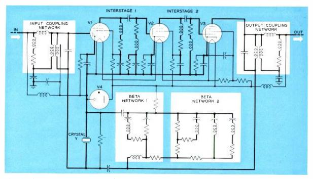
The circuit used for the transatlantic repeaters. It compares with the Key West-Havana circuit except that the present design has a more elaborate
