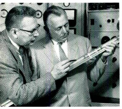
W. A. Klute (left) and W. M. Bishop examine an amplifier section. This view shows the unsheathed amplifier with adjacent sections attached to each other; they are connected electrically by bus tapes.
