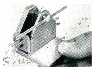
The torsional transducer: torque is applied to the arm on the free end of a germanium crystal; the other end is firmly cemented to a backing plate.
