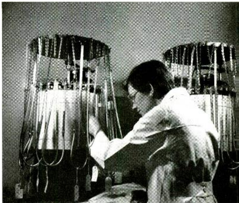
Mrs. B. B. Loeffler checks and records the oxygen uptake of a sample of polyethylene with a protectant added. By matching the level of the mercury in the tubes, she can determine how much of the oxygen in the tube has been absorbed by the sample, also enclosed in the tube. Bath behind the glass tubes contains heated silicone to keep the samples at a constant temperature.
