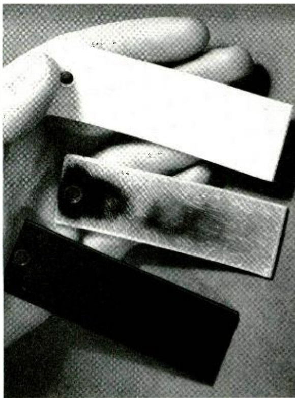
These small samples of polyethylene with various additives were exposed at Yuma, Arizona, for about 3½ years. Severe cracking is evident in the two samples, center and top, containing, respectively, 1 per cent of a blue organic dye and 2 per cent zinc oxide. The sample at the bottom, containing 2 per cent carbon black, shows no cracks and has retained its original flexibility.
