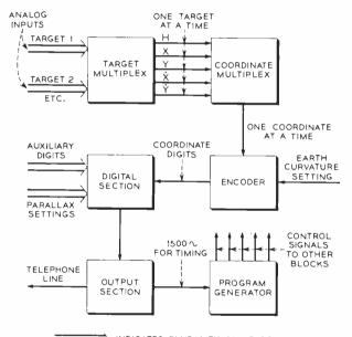
Fig. 3 — Block diagram of AN/TSQ-7 transmitter.
