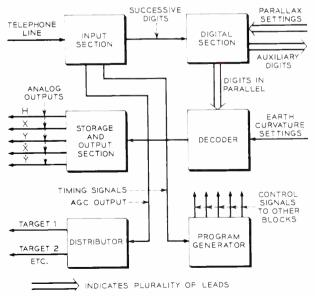
Fig. 4 — Block diagram of AN/TSQ-7 receiver.
