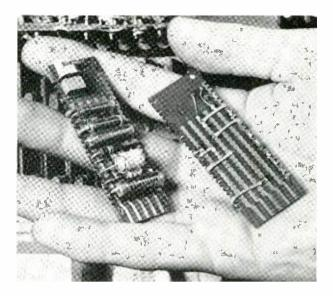
In antiaircraft fire coordination systems, the data obtained by radar must often be transmitted for long distances to processing centers. Laboratories' engineers have developed transistorized units to do this rapidly and accurately over telephone circuits. This military equipment converts analog data to digital form for transmission and then returns the data (binary numbers) to the original analog form at the receiving end of the system.
