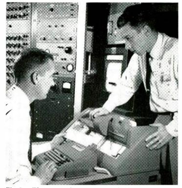
Fig. 3 — The system elements: racks of tube panels extend to left; rack at center contains control elements; author (left) and R. R. Spiwak at recording section of the equipment in the foreground.
