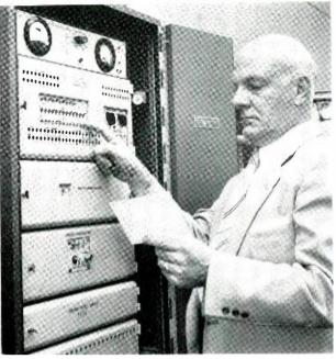
Fig. 5 — The author sets in parallax figures on the receiver of the AN/TSQ-7 system equipment.
