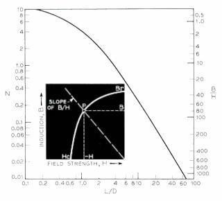
Fig. 1 — Plot of relationships of B/II, L/D and N. Inset shows part of typical demagnetization curve.
