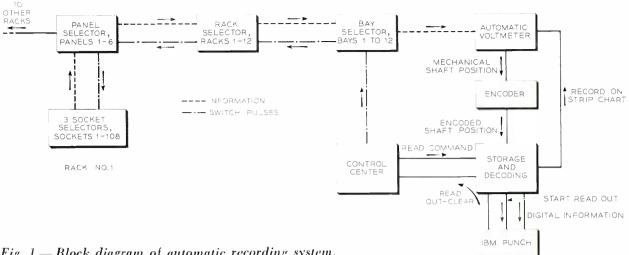
Fig. 1 — Block diagram of automatic recording system.
