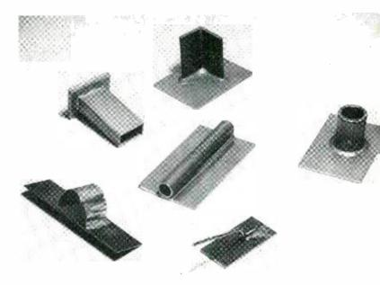
Fig. 5 — A number of constructions are possible with the application of the recently evaluated procedure for the efficient soldering of aluminum.
