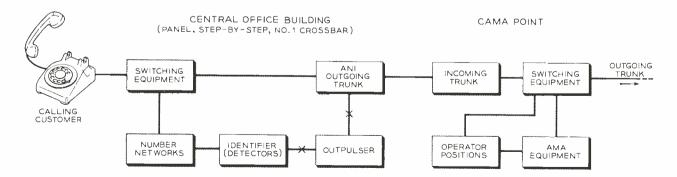
Fig. 2 — Diagram of ANI equipment in central office and connecting equipment at CAMA point.
