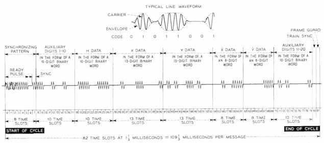
Fig. 2 — Typical transmitted AN/TSQ-7 message. Inset shows the line waveform for eight digits.
