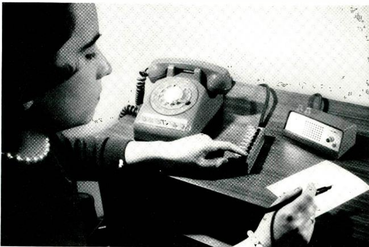
Fig. 1 — Speaker phone-equipped key telephone with six push-buttons and additional “pad” of keys.
