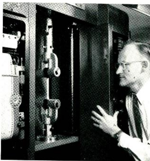
Fig. 5 — R. R. Hart observes a tensile test in progress in the automatic Instron testing machine.
