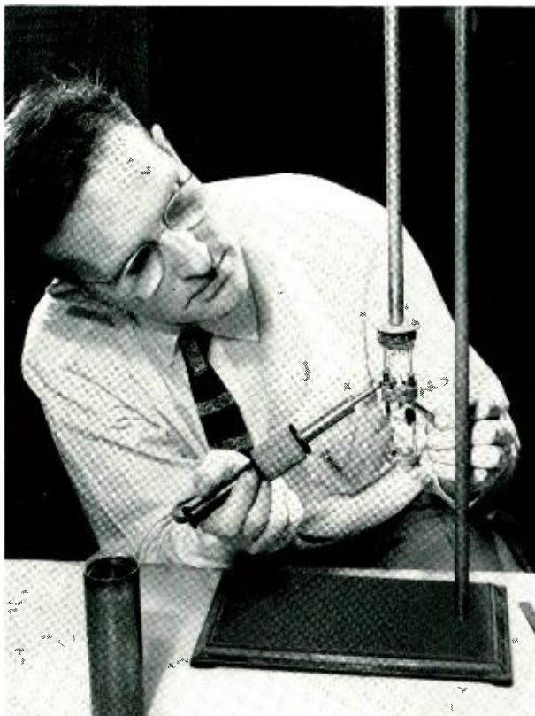
Fig. 3—D. F. Gibbons secures test leads for low temperature elasticity measurements.
