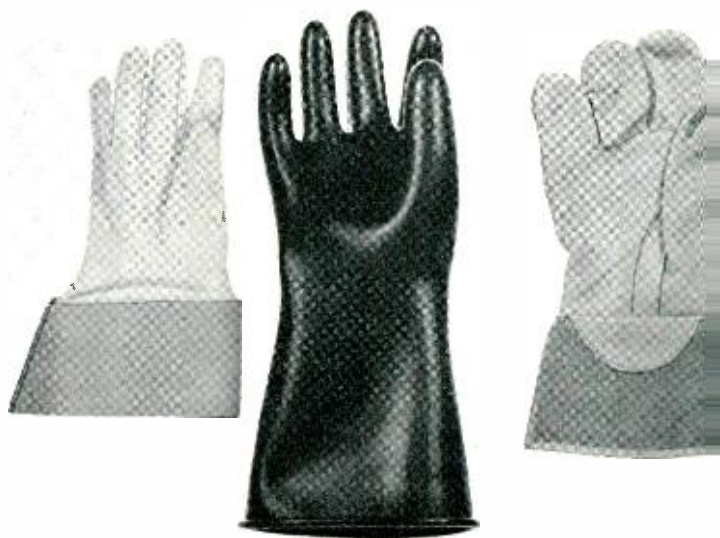
Left, fabric liner glove worn beneath rubber glove; center, lineman's rubber glove; and right, leather protector glove worn over rubber glove.
