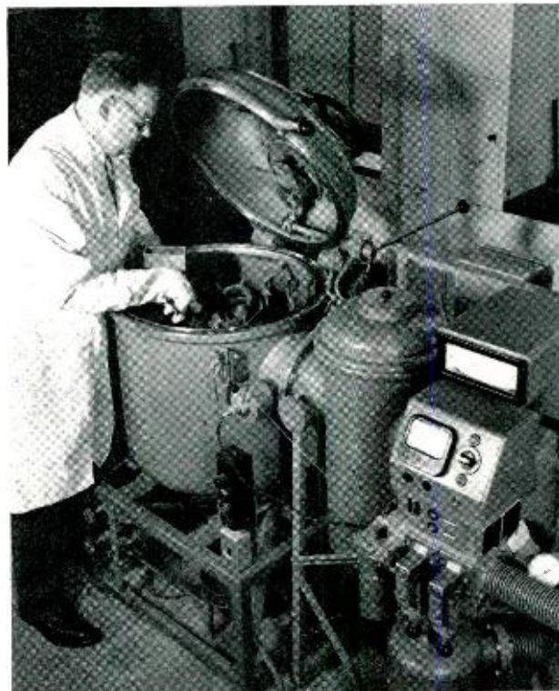
Fig. 4 — P. H. Schmitt removes the mold from the high vacuum furnace.
