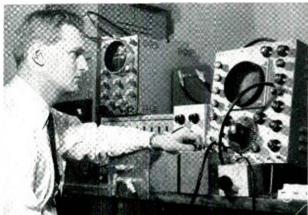
Fig. 8 — A. G. Chynoweth measures Barkhausen jumps in G.A.S.H. with equipment affording high electrical resolution.
