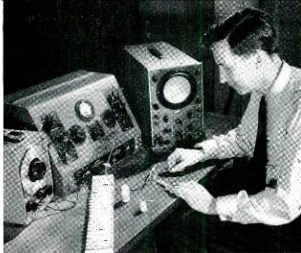
Fig. 4 — B. T. Matthias puts silver paste electrodes on a crystal preparing to test it for ferroelectricity. In this way, he recently found that guanidinium aluminum sulphate hexahydrate, a substance discovered by Ferraboschi in 1908, was ferroelectric.
