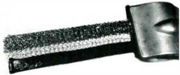
Fig. 2—The new wire-mesh and conducting rubber microwave seal.
