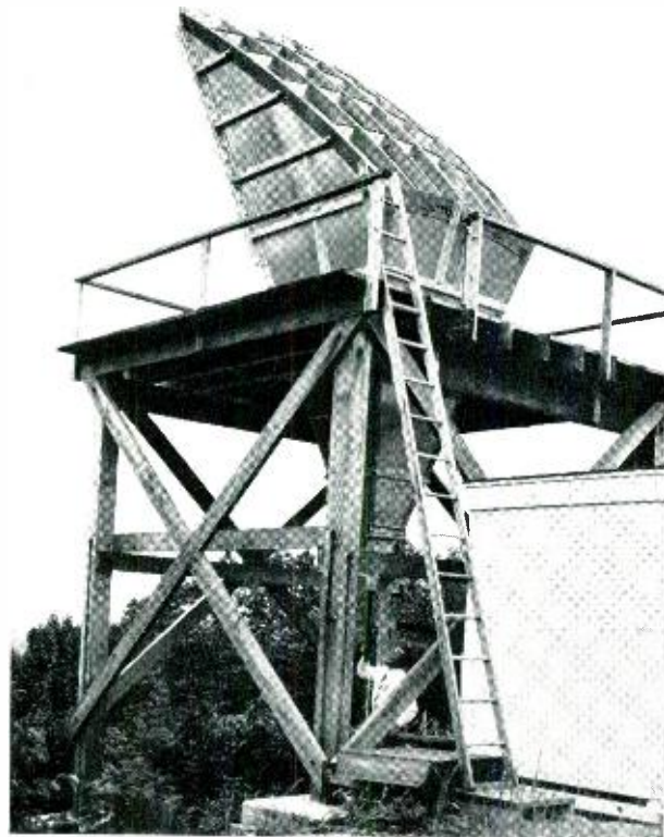
Horn-reflector antenna that is used for making tests at the Holmdel Laboratory.
