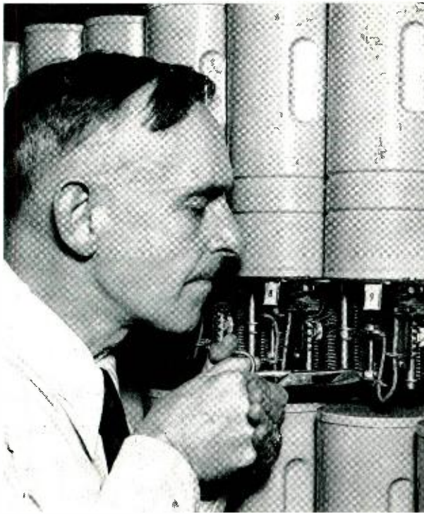
The author snips a worn spring from a wiper in service in the Laboratories.
