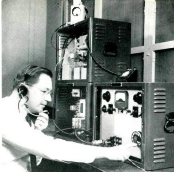
Fig. 1 — E. J. Henley operates the control unit of an emergency radio telephone terminal during Laboratories field tests of the system.
