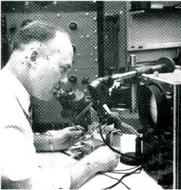
Fig. 6 — R. L. Johnston bonding lead to n-p-n junction bar in micromanipulator. Oscilloscope at right tells when correct position for bonding is found.
