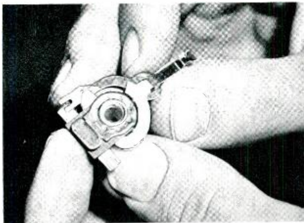
Fig. 2 — A replaceable spring is inserted into a wiper assembly.
