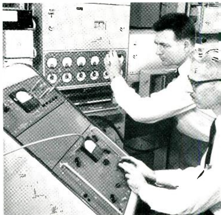
Fig. 4—W. Freeman (front) of the A.T.&T. Company and the author calibrating the pilot indicators.
