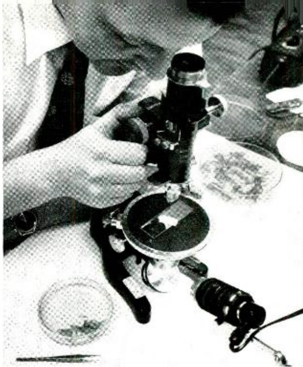
Fig. 11 — A barium titanate crystal being examined with a microscope in order to determine the domain structure.
