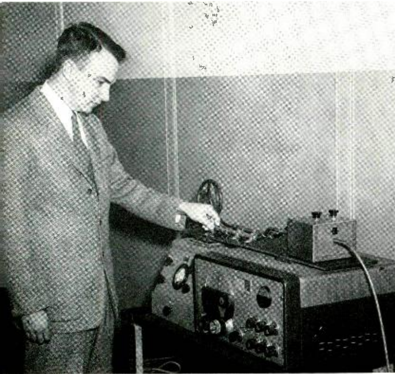
J. T. Maupin adjusting "line-stretchers" on precision phase-shift difference measuring equipment.
