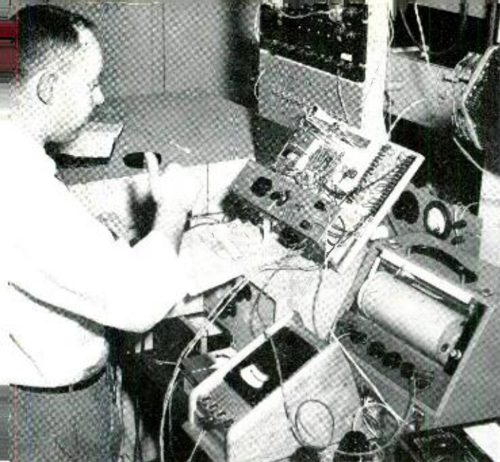
Fig. 6—Tests on a power supply are made using a series current regulator. J. J. Wilson checks the circuit.
