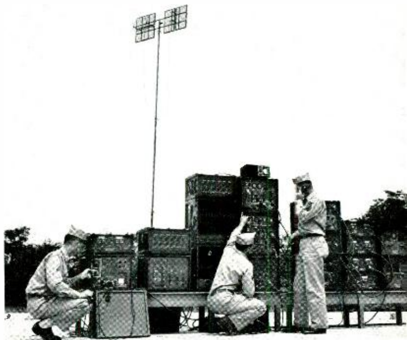
Fig. 3 — For purposes of demonstration, complete four- and twelve-channel terminals and radio equipment are here assembled with AN/TRC-24 antennas in background. In operation, units would normally be under protective cover.
