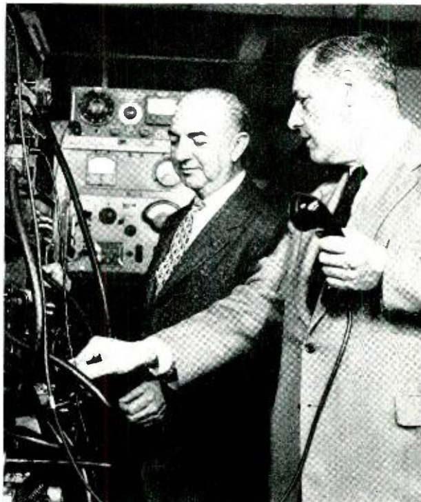
Fig. 5 — At the Marion Shops of the Western Electric Company, the author (left) and R. R. Andres inspect twelve-channel terminal equipment.
