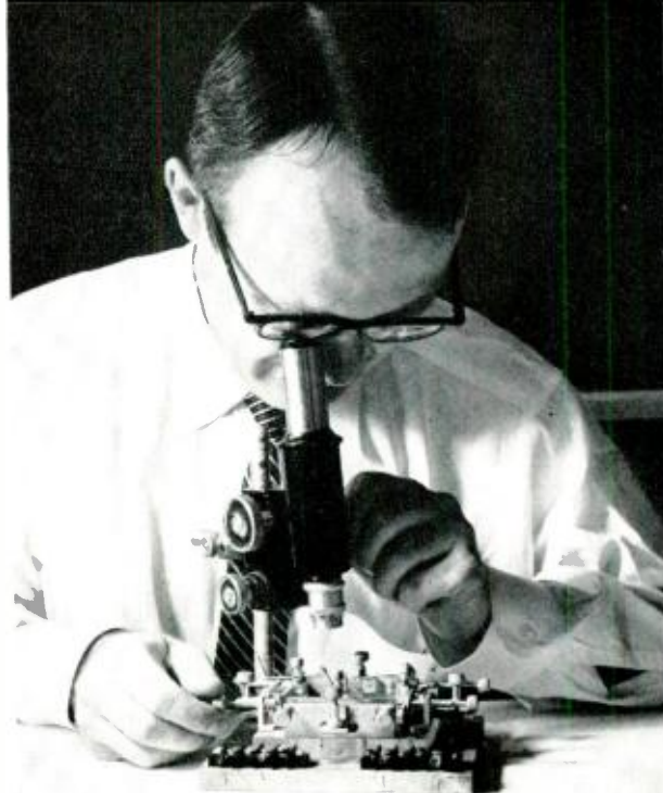
Fig. 6 — J. K. Galt using micromanipulator to bend a metal whisker on a specimen.
