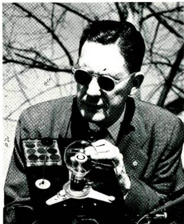
D. F. Ciccoella compares the electrical output of the battery with the total energy available from the sun as measured by a pyrheliometer.
