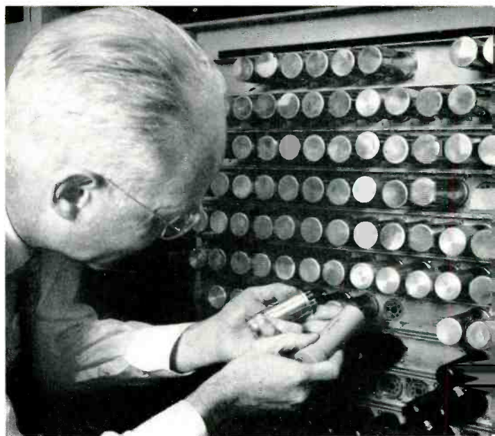
Fig. 4 — E. J. Donohue replacing a 149A transistor amplifier (left hand) with a 100A test set in a Bell Laboratories' card translator.
