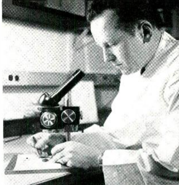
Fig. 4—W. Weigman assembling a field-effect transistor by means of a special jig.
