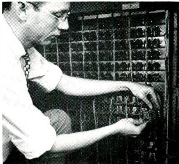
Fig. 2 — The author inserting a 680A input transformer into a Bell Laboratories' card translator.
