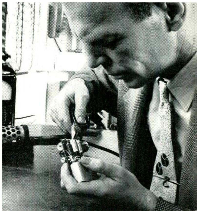
Fig. 1—F. E. Ladd wiring the components in a packaged amplifier before it is embedded in plastic.
