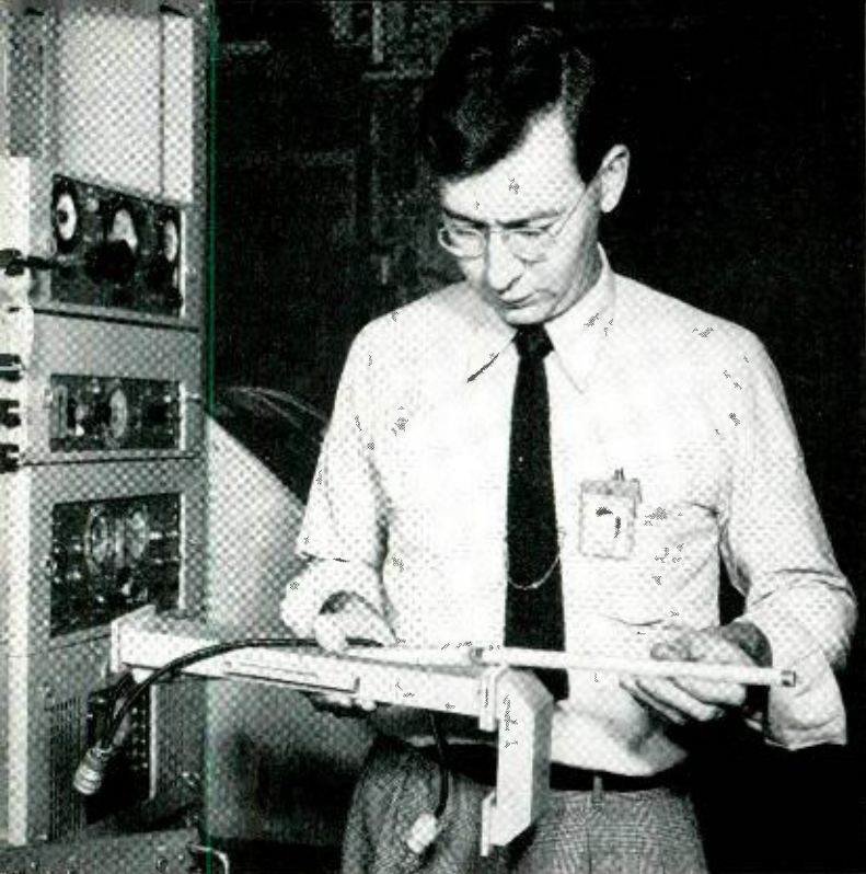
Fig. 3 — The author inserts a fluorescent tube into its special diagonal mounting in the waveguide. This mounting matches the waveguide and produces optimum noise power.
