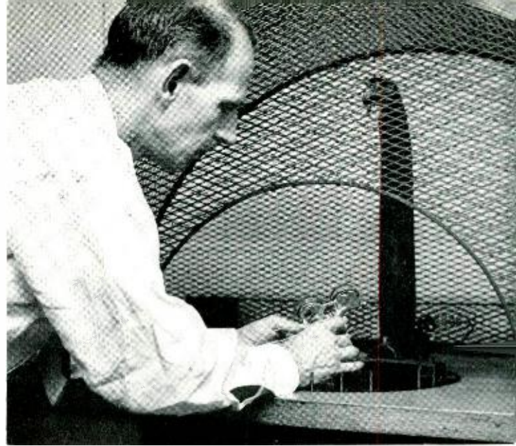
Fig. 1 — W. Kalin placing a telephone ringer in an integrator of earlier design.
