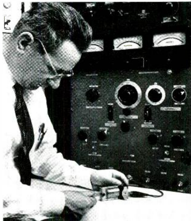
Fig. 7—B. Stauss preparing an AG relay for static flux measurements.
