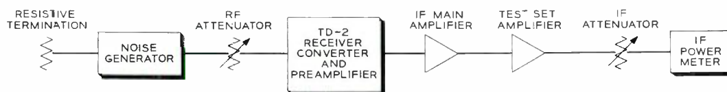
Fig. 2 — A block diagram of a typical test set-up using the noise figure test set.
