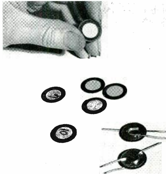
Fig. 2—Experimental discs with electrodes in place (top) and completed discs with terminals attached (bottom).
