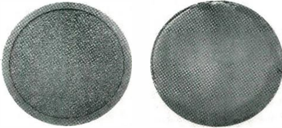
Fig. 8—Varistor discs as formed by a rubber-faced punch (left) and a steel-faced punch (right).
