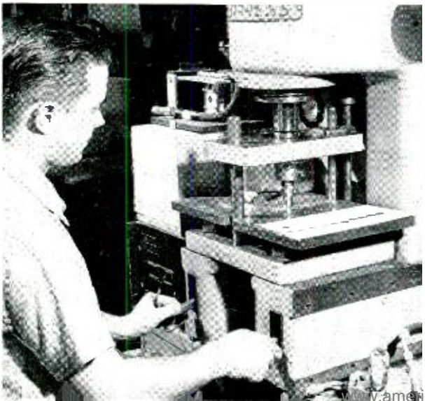
Fig. 6—E. B. Berry operating a press used to form varistor discs.
