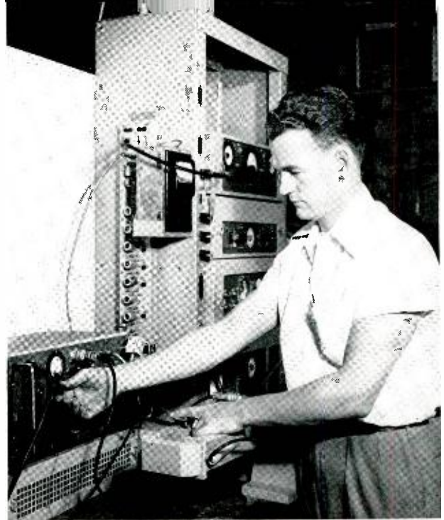
Above — G. D. Brown using the test set to measure the noise figure of a TD-2 converter-preamplifier. The fluorescent tube noise source in the foreground is stored in the test set compartment.
