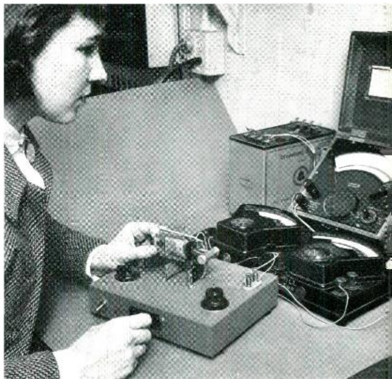
Fig. 3 — Mrs. K. R. Randall measuring coercive force of magnetic parts of the AG relay.
