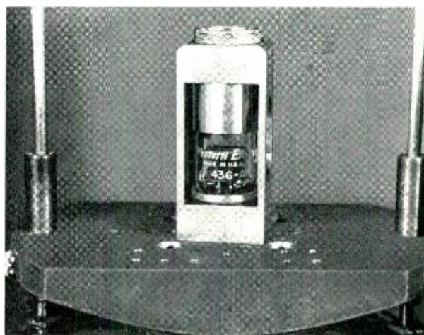
Fig. 3 — A closeup view of the shock test table with a 436A electron tube in place.
