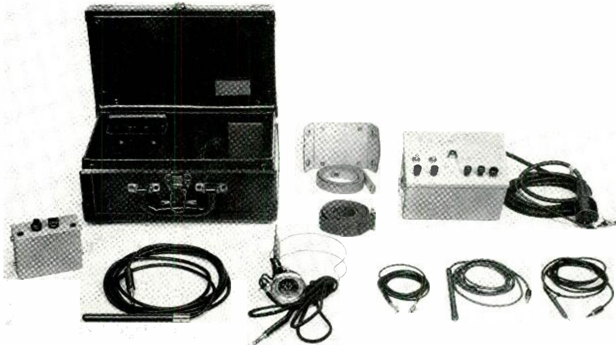
Fig. 3—The 1A fault locator test set showing the component parts. The carrying case holds all of the elements for easy transportation.
