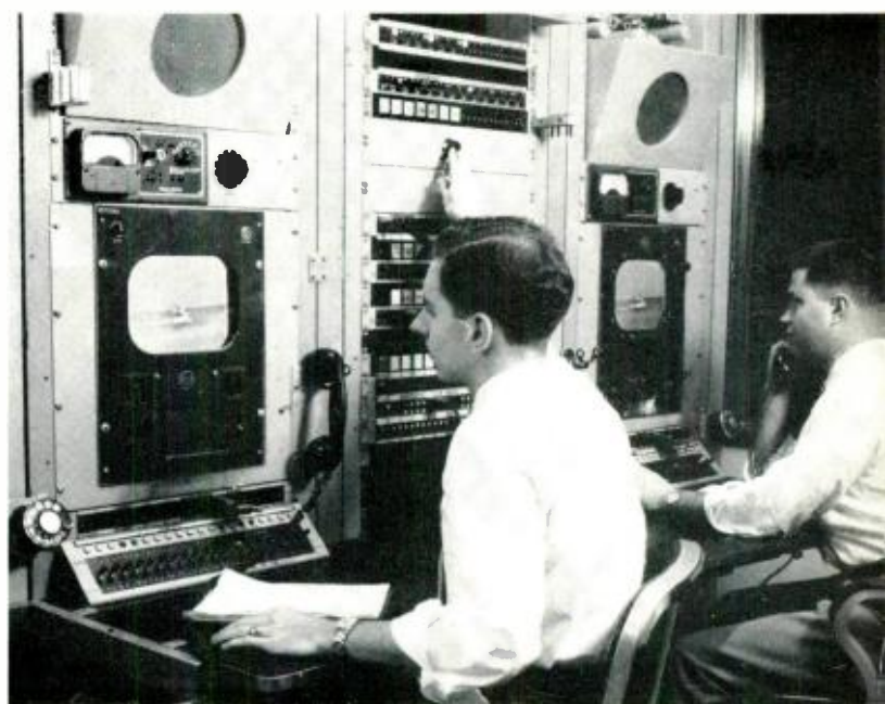
Fig. 3—W. G. Goetz and R. L. Goes monitor television picture quality at the New York Long Lines building.
