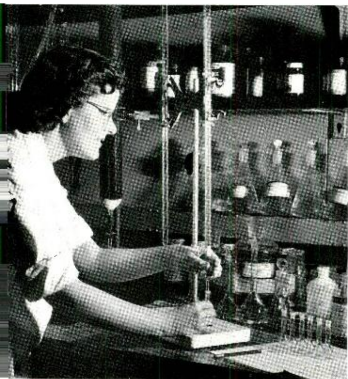
Fig. 2—Preliminary to the actual analysis, a calibration curve of light intensity versus concentration is prepared. Miss Mary Campbell here transfers measured amounts of an arsenic solution to volumetric flasks.
