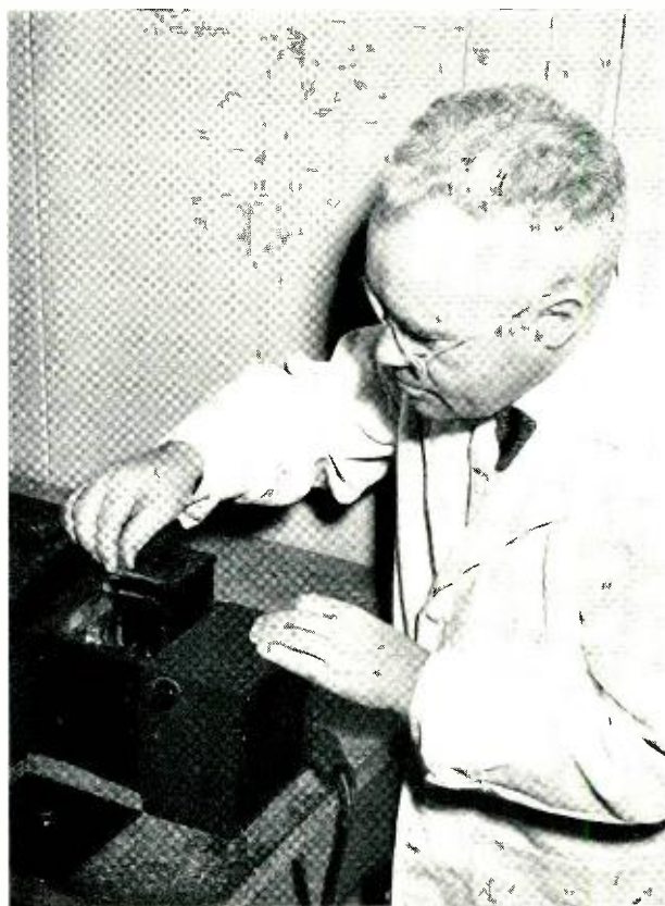
Fig. 4—The test solution in an absorption cell is next placed in a spectrophotometer. The amount of light that can pass through this absorption cell is a measure of the concentration of arsenic in germanium dioxide.
