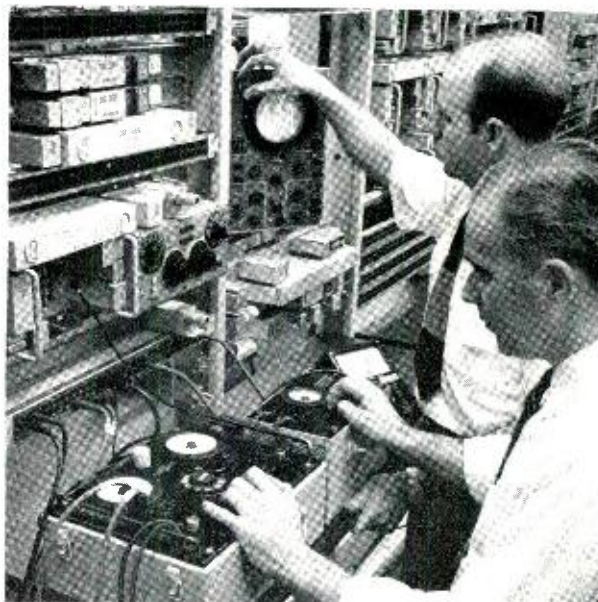
Fig. 1—J. M. Wiswall (right) and E. M. Hoffman testing the pulsing characteristics of the new single-frequency equipment.
