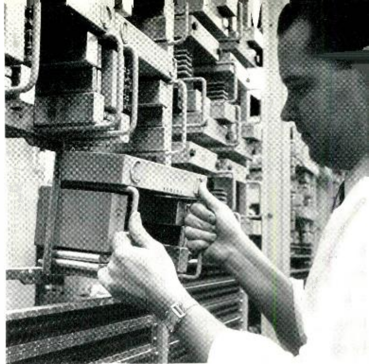
Fig. 2—R. E. Staehler pulling a single-frequency unit out of its frame to illustrate the rapidity of maintenance changes.
