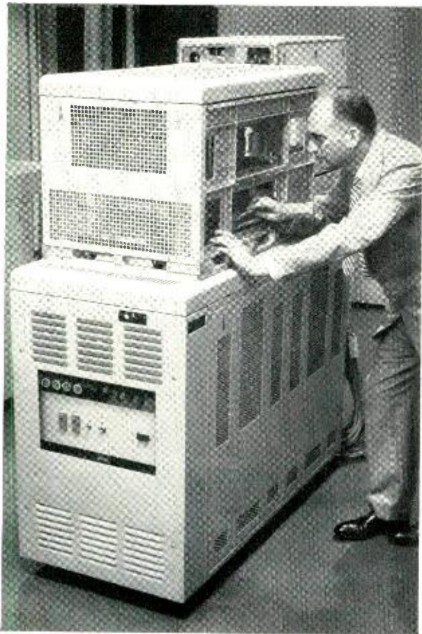
Fig. 1—The author inspecting a card translator, which is the heart of the equipment necessary for the automatic alternate routing of traffic.
