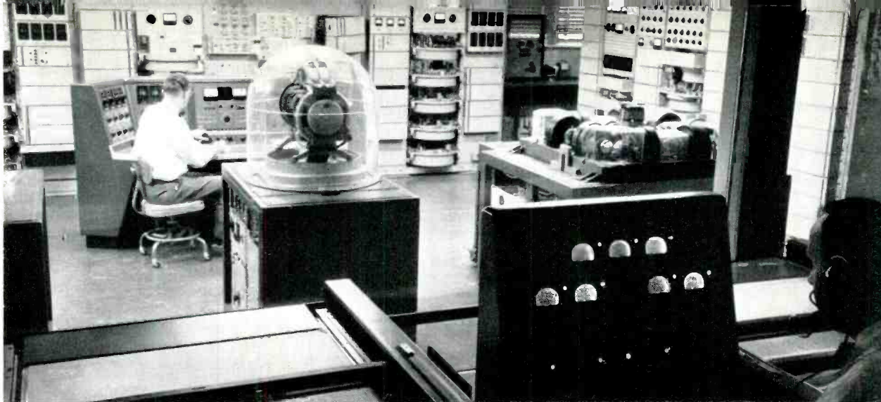
J. F. Yost, left, and J. J. Oestricher, extreme right, introduce typical flight problems into electro-mechanical equipment which simulates Nike.
