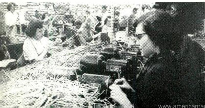
Wiring and assembly operations in the production of Nike ground guidance equipment at a Western Electric plant.
