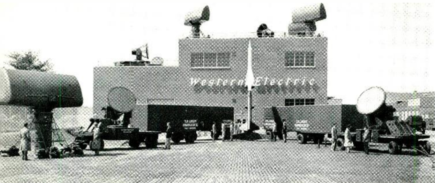
Check-out tests of Nike I ground equipment performed by the Western Electric Company, prior to delivery to the government.
