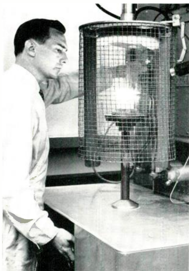
Fig. 1 — P. M. Ness working with a radio-frequency induction heater.
