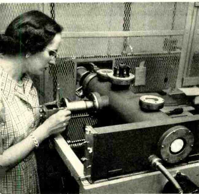
Fig. 3—Mrs. M. H. Read adjusts a sample in the electron diffraction camera.
