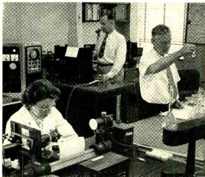
Miss B. E. Prescott measures the density of a spectrum line on a photographic plate, while W. Hartmann positions a sample in the arc stand of the spectograph, E. K. Jaycox is preparing a sample for analysis.
