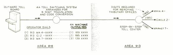
Fig. 5 - Typical three-digit combinations as they might be dialed by an operator and as they might be converted by a 4A system.
