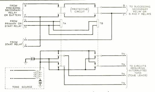
Fig. 4 - The TA-TB secondary relay supplies interrupted tone only.
