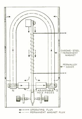
Fig. 5 – Schematic magnetic circuit of the 239-type relay.
