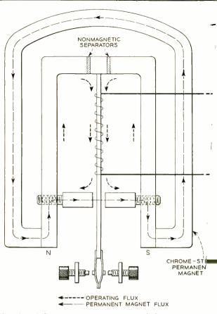
Fig. 4 – Schematic magnetic circuit of the 206-type
