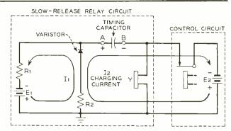
Fig. 8 – Timing circuit for slow-release relays showing path of charging current. Operating current for relay Y from voltage  $E_2$  is not shown.
