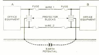
Fig. 2 – Schematic representation of a simple telephone circuit, with protective arrangements and a high earth potential difference.
