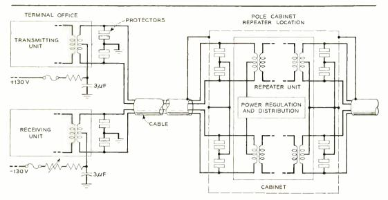
Fig. 1 - Simplified schematic showing arrangement for supplying power over the cable to a pole-mounted N1 carrier repeater.
