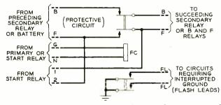
Fig.  $2 - The \ \mathbf{FC}$  secondary relay supplies interrupted ground only.
