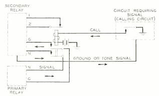
Fig. 6 – The start relay connects primary and sccondary relays when called by associated circuit. Leads 1 and 2 are normally closed to prevent the idle secondary relay from operating the protective circuits.
