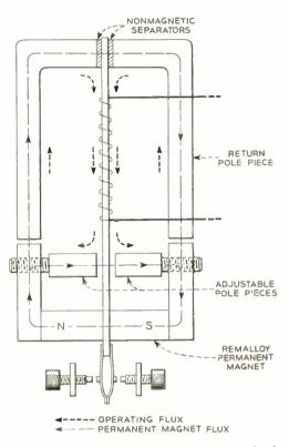
Fig. 6 – Schematic magnetic circuit of the 280-type relay.
