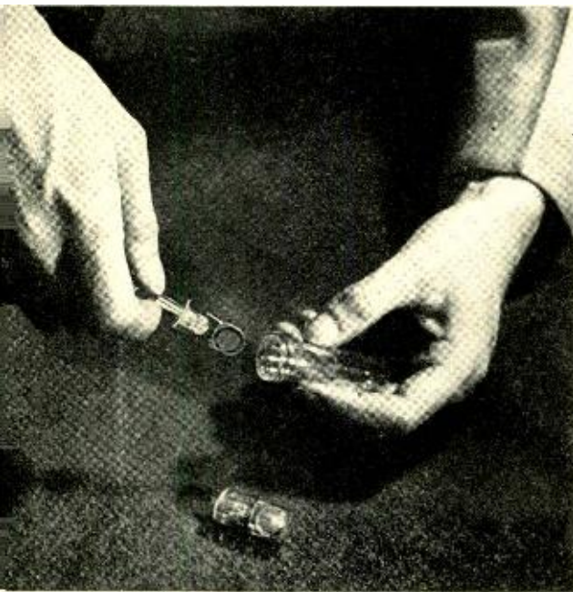
Fig. 1—Precise high-frequency crystal unit. The unit is sealed in the glass envelope. A completed unit is shown in the foreground.
