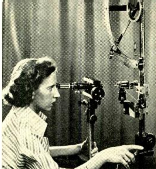
Fig. 6 – With pull machine set up to measure load, Dorothy Lapidus observes armature displacements corresponding to various restoring spring forces or loads.
