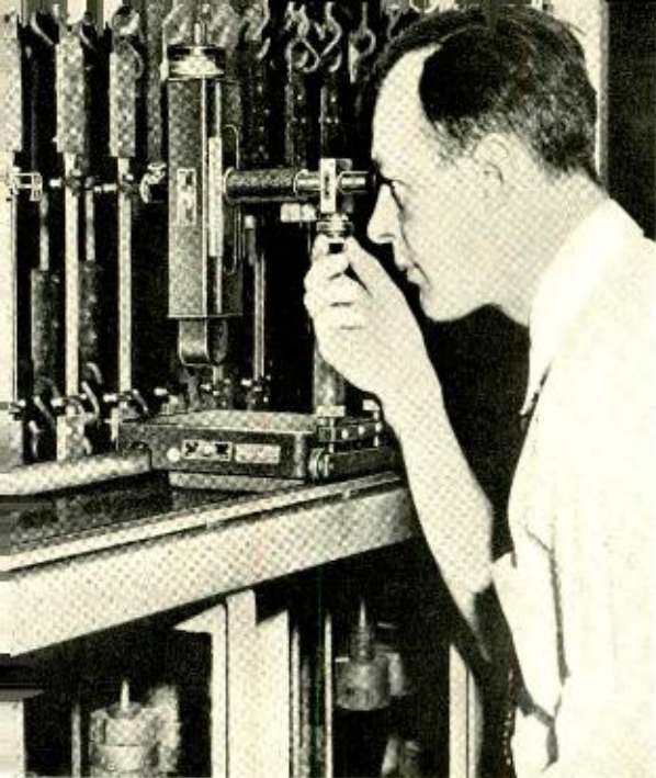
Fig. 2—J. P. Ahrens making measurements using the new 10:1 mechanical extensometer and cathetometer on a group of specimens.
