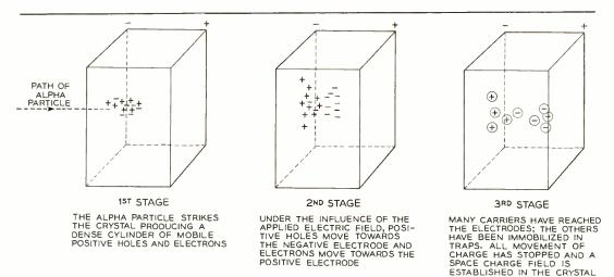
Fig. 1-Simplest case of alpha bombardment conductivity.
