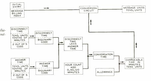
Fig.  $1-B l \circ c k$  diagram of the computing operations.
