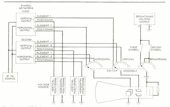
Fig. 8–A simplified diagram illustrating the use of the switch assembly in applying the wave forms for a single and double-element character to the CRO tube.
