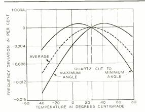
Fig. 3–Temperature characteristics of a typical crystal used in repeater oscillators.
