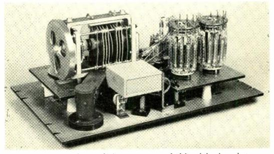
Fig. 1–Interior of the bridge. Standard capacitor  $c_s$  is on the left and decade conductances  $c_s$  on the right.
