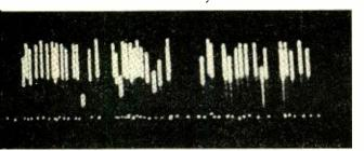
Fig. 8–Pulses from a germanium n-p junction bombarded by monoenergetic alpha particles. With a few exceptions, most of the pulses are the same height.
