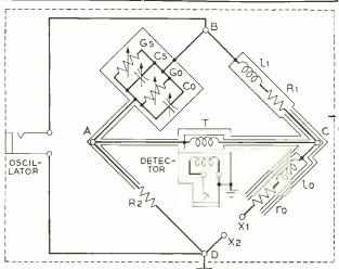
Fig. 3—The complete schematic of the bridge, including the shields.
