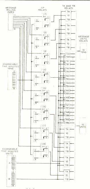
Fig. 2-Simplified schematic of the circuit that converts from chargeable time to message units.
