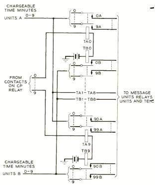
Fig. 3–Schematic showing the arrangement of the TA and TB relays associated with each CP relay.
