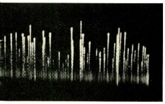
Fig. 5–Pulses from a diamond crystal bombarded by monoenergetic alpha particles. Observe the scatter in pulse heights due to nonuniform response.
