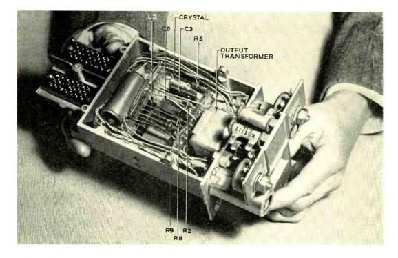
Fig. 4-The oscillator components are mounted on a sub-assembly panel along with other components. The top of the panel is shown above and the back at the bottom.
