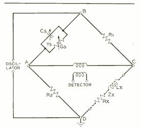
Fig. 2–The basic circuit is that of a Maxwell bridge.
