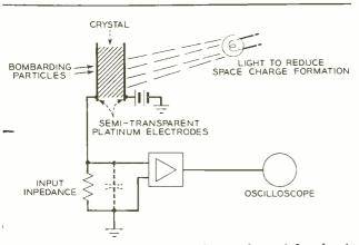
Fig. 2-Typical schematic for studies of bombardment conductivity in insulating crystals.
