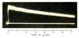
Fig. 7-Sixteen superimposed pulses from alpha particles striking a germanium n-p junction shown on an expanded time scale. The very fast rise time indicates that the electrons and holes produced by the bombardment are swept across the junction in a time less than  $10^{-8}$ seconds.
