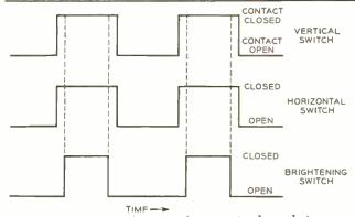
Fig. 7–A diagram showing the magnitude and time relationship of the open and close times of the horizontal, vertical, and brightening switches.
