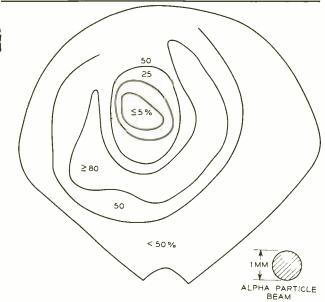
Fig. 6–Plot of the counting efficiency in per cent of a large flat diamond when bombarded by alpha particles. Such wide variations in sensitivity in different parts of a diamond are usually encountered.
