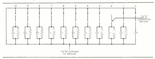
Fig. 4–A developed circuit of the decade conductances. Rotor switches connect all resistancecapacitance networks to ground except one, for each position of the decade dial.
