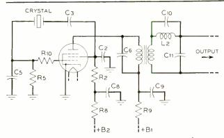
Fig. 2–Circuit of the 304 kc (group unit and repeater) oscillator.
