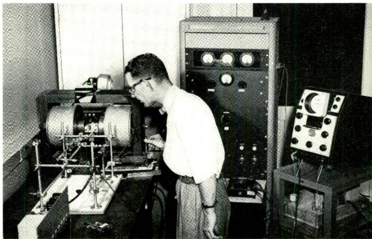
Fig. 4—R. F. Heck adjusts the electromagnetic field with respect to the spatial harmonic amplifier, in order to make the axial slots in the tube accurately parallel to the direction of magnetic field. This provides for a maximum of electron transmission.
