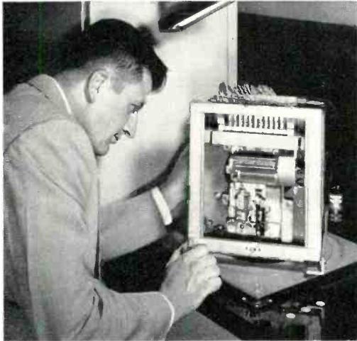
Fig. 2—By tipping up the perforator, sliding back and then rotating its mounting, its under-surface is exposed for inspection or adjustments.
