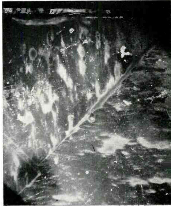
Fig. 3—Powder pattern formed at the corner of a hollow rectangle, showing the domain boundary. The enlargement of (b) is shown at the right.
