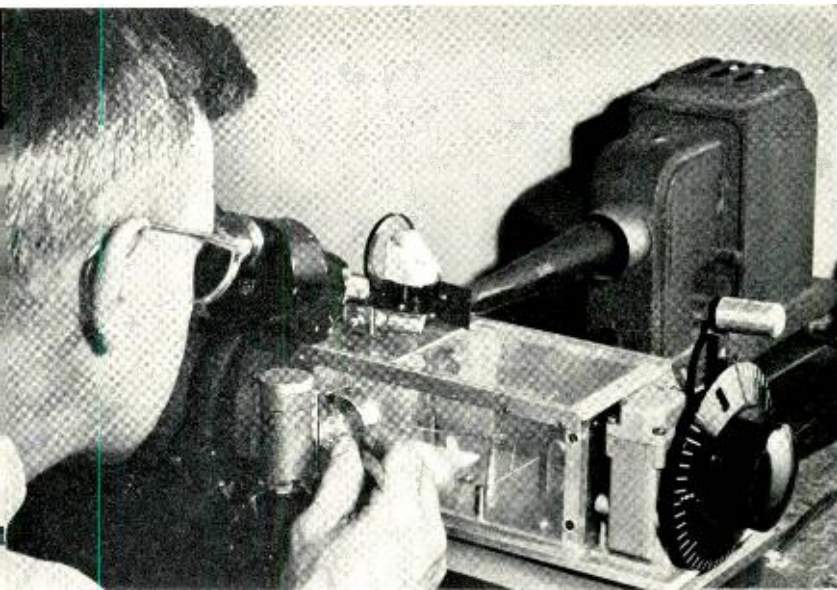
Fig. 1—G. E. Reitter loads a scale pan with the aid of a stereomicroscope.
