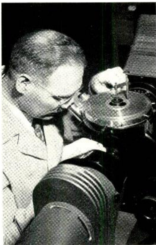
Fig. 10—The metallograph used in the examination of opaque specimens.
