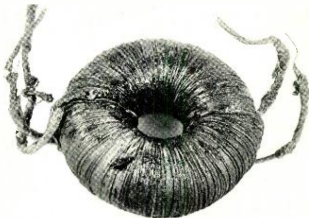
Fig. 3—One of the 501-type loading coils designed by Warren and first used on the open-wire circuits between New York and Chicago.
