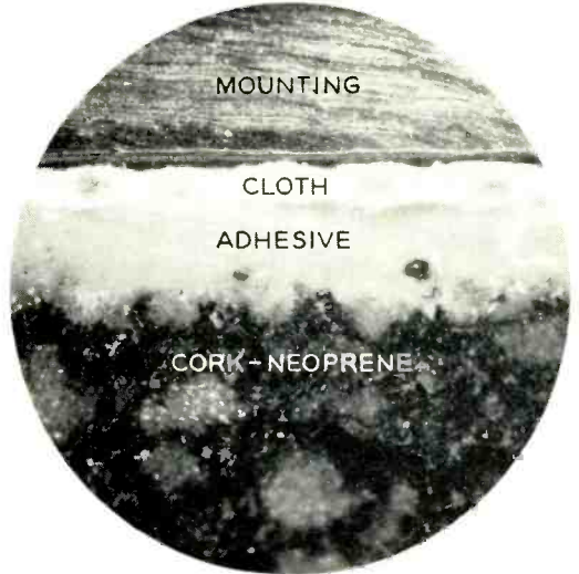
Fig. 12—Micrograph of a section of cloth backed adhesive coated cork-neoprene (50 diameters).
