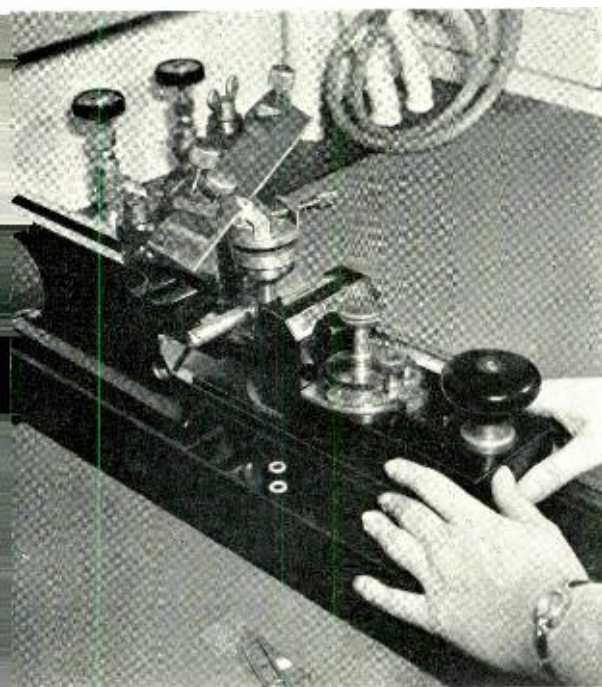
Fig. 2—The microtome in use, slicing a thin section of polyethylene tubing.
