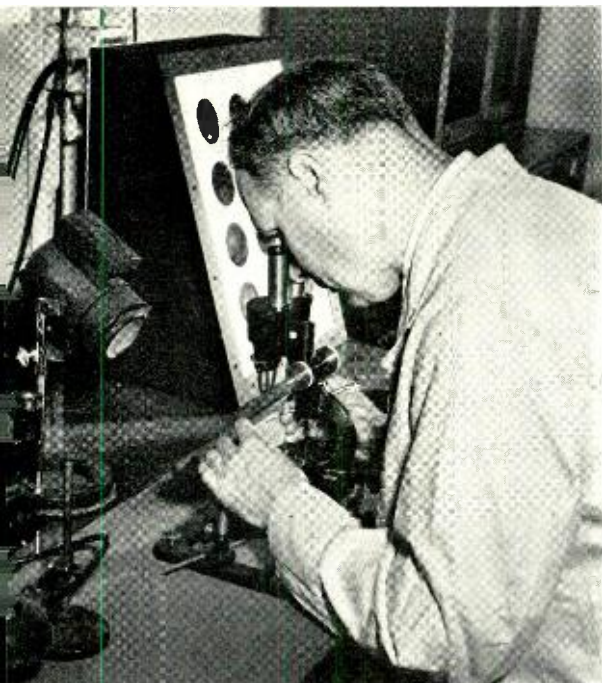
Fig. 1—The first step in microscopy, a cursory examination, is made with a low-power binocular microscope.
