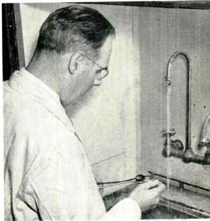
Fig. 6—The specimen is finally etched to develop grain structure.
