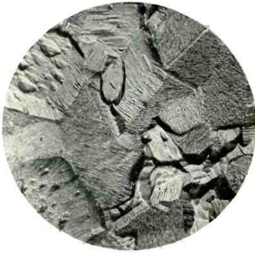
Fig. 11—Micrograph of annealed pure nickel shows the influence of oblique illumination on resolution (750 diameters).
