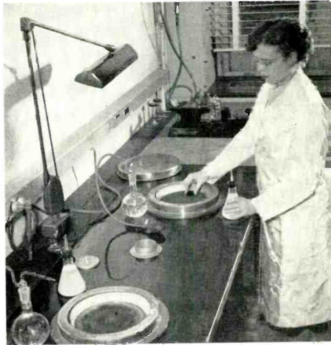
Fig. 5—Final lapping is done on a rotating cloth covered wheel charged with alumina.
