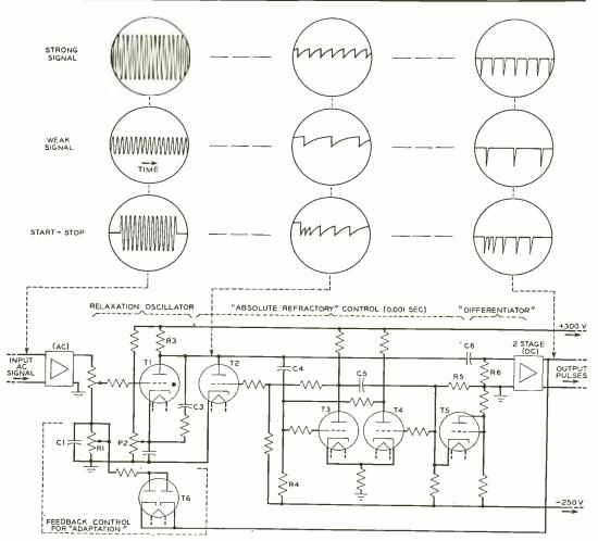
Fig. 2-Schematic of the analog "hair cell" pulsing circuit, with illustrations of several sample wave forms of the operating voltages.
