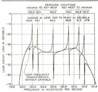
Fig. 2-Measured transmission characteristics of test frequency loop circuit showing the crystal peaks and dips. Tube performance of a particular repeater is indicated by the difference between its peak and closely adjacent dip loss.
