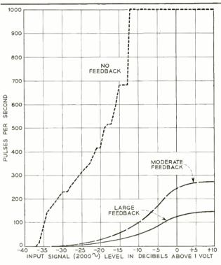
Fig. 3–Response characteristics of the analog "haircell" pulsing circuit.
