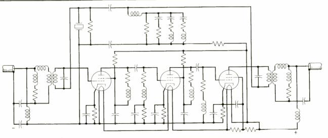
Fig. 1–The repeater circuit.
