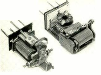
Relays play an important part in telephone communication, and while many of them do a routine job of closing and opening circuits, others must perform their tasks in a certain way or under limitations that require special consideration in their design. Such a relay is the recently developed 268 type, shown in Figure 1, to replace the 207type relay.
