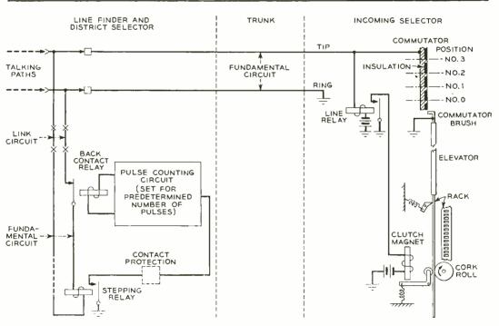
Fig. 2-Schematic of the fundamental circuit of the panel system. The stepping relay is shown at the lower left.
