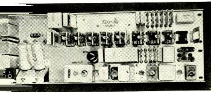
Fig. 3—Single-frequency signaling circuit equipment.
