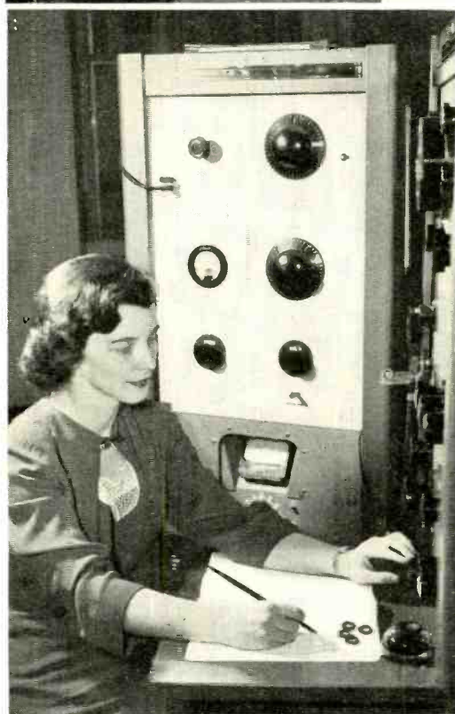
The fired parts are carefully checked for dimensional accuracy. Here F. R. Monforte is measuring the inside diameter of a toroidal core that is to be used in a retardation coil or transformer.
