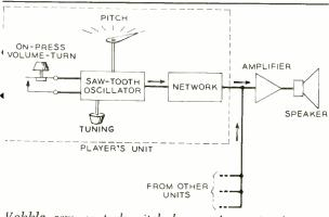
Vobble arm controls pitch by varying potentiometer. 'wo other potentiometers control volume and tuning. arrangements could be inexpensively built of standard radio parts. Working for two nights in his cellar, Meacham produced the instrument.
