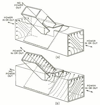
Fig. 5-Perspective drawing of the waveguide hybrid unit showing its effect on entering waves polarized in two directions.
