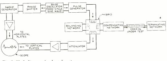
Fig. 2-Block diagram of pulse echo set.
