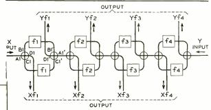
Fig. 3–Block schematic of the chain of separating or combining filters.
