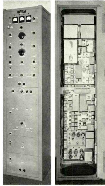
Fig. 2-The Western Electric LD-R1 receiver.
