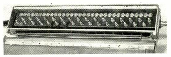
The new 16-pair gas-tight protected terminals (coded NC-16).
