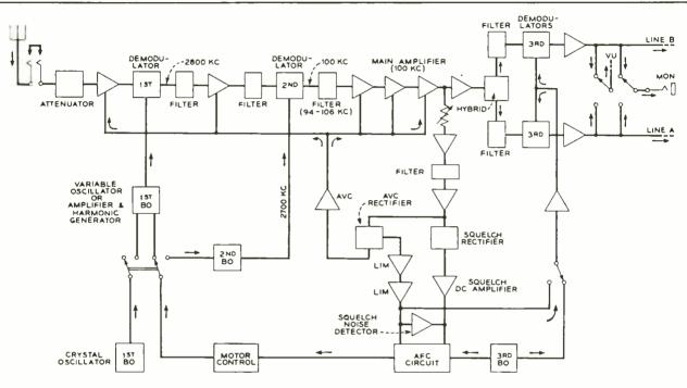
Fig. 1-Block schematic of the LD-R1 single sideband radio receiver.
