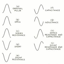
Fig. 6–Reflections or echoes resulting from various types of irregularities.
