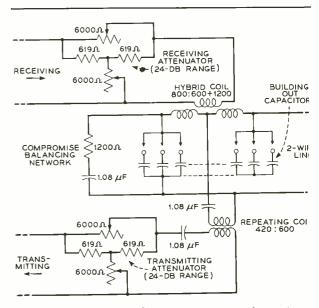
Fig. 1–Schematic of the new miniature four-wire terminating set.
