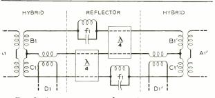
Fig. 2-A wire circuit analogy of the chain of a separating or combining filter unit.
