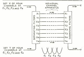
Fig. 1—A set of four incoming channels is connected to one end of the separating filter chain, and another set of four to the other end, and the eight individual channels are separated by the filter. In a similar manner, the chain of combining filters takes eight individual channels and forms two groups of four.
