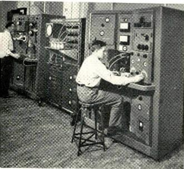
Fig. 1—Phase, delay and transmission sets in the new cabinets in the filter laboratory at Murray Hill. Left to right, F. W. Webb, R. J. Kirkpatrick and D. A. Alsberg.
