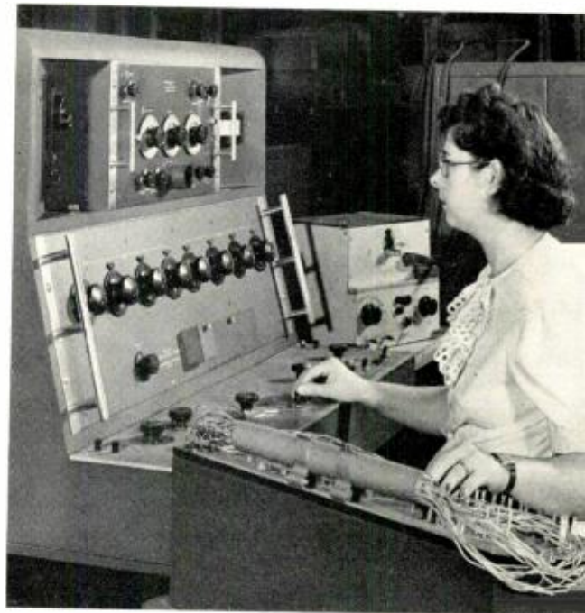
Fig. 1.—The balanced Maxwell bridge mounted in a loading coil test set in service at the Hawthorne plant of the Western Electric Company.
