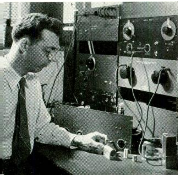
Apparatus used in the laboratories for measuring sound transmission in solids at ultrasonic frequencies.
