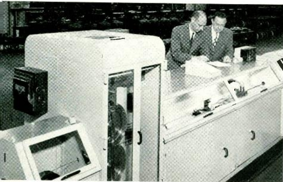
A. S. Windeler, Laboratories engineer stationed at Point Breeze, confers with H. R. Longfellow, an engineer of Western Electric. Machine in foreground makes coaxial tubing: first it snaps insulating discs onto the central wire, then forms a copper tape around the discs, and finally wraps on a double layer of steel tape.
