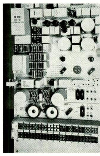
Fig. 5–One channel terminal with its oscillator and common monitoring and testing equipment
