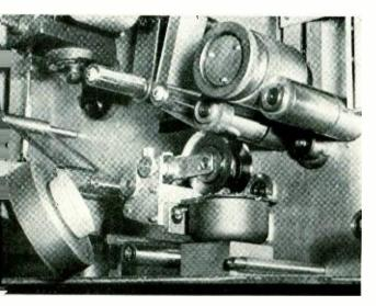
Fig. 6—The two lubricated cutting wheels press the paper against the hardened steel rolls, scoring the paper sufficiently to cause separation. A slit roll is held, left, with the unplated margin evident
