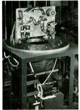
Fig. 5–Vacuum vapor-plating machine with bell jar and side panel removed. The plating occurs in the upper section normally covered with the evacuated bell jar. Below are located oil diffusion pumps, transformers, speed control and the water-cooling coils
