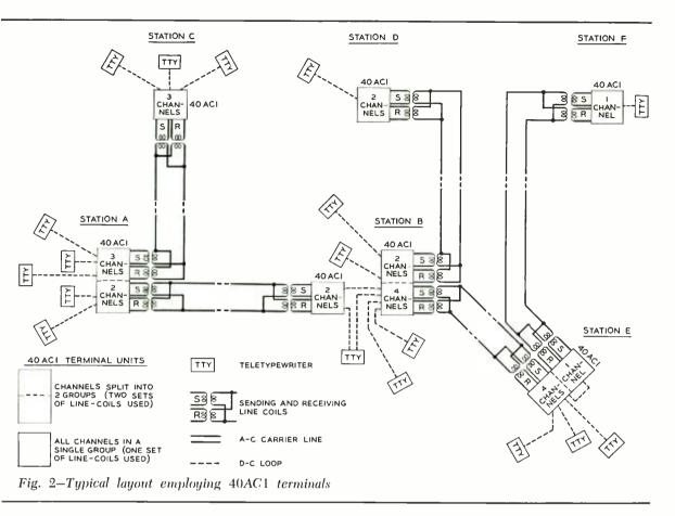
and more flexible in application. To make it adaptable to isolated locations, provision is made for its entire operation from commercial a-c power but, if preferred, the telegraph currents for the loops and even the plate current may be supplied from external d-c sources. Power to heat the vacuum tubes, however, must be derived from an a-c source. The testing equipment is an integral part of each system so that very little auxiliary equipment is needed.
