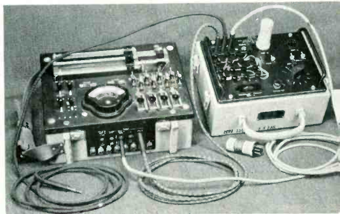
Fig. 6—A test set-up for a non-standard relay
