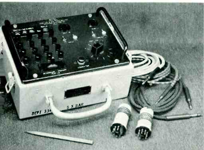
Fig. 3—The J94725A test set for type 275 and 276 relays. In the foreground are a 276-type relay at the left and a 275 type at the right
