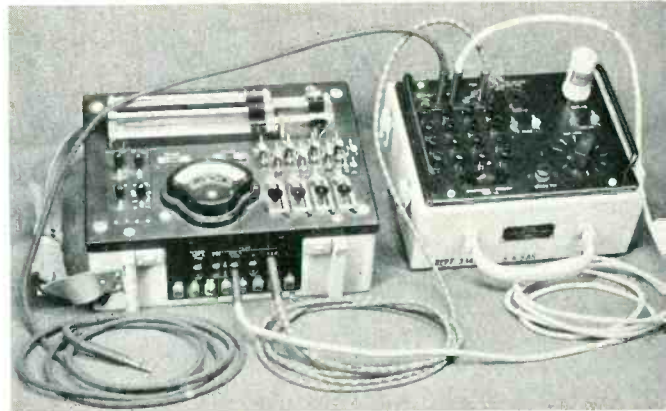
Fig. 4—A No. 35 test set at the left connected to the relay test set by the cords that are provided with the latter set
