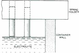
Fig. 7-Level indicator. The mean length of the pins corresponds to the spring length desired after pointing. The liquid is raised until it wets the longer pin only. The pins differ in length by only a few thousandths of an inch
