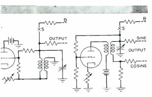
Fig. 1–Two forms of the start-stop oscillator circuit
