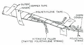
Fig. 2-Section of video pair showing construction details of the various elements
