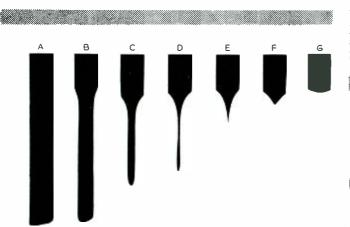
Fig. 3-Photomicrographs of 0.005 inch tungsten wires at successive stages of anodic solution. Contour F is most representative of those used in point contact rectifiers. Magnification-100X
