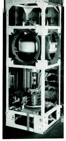
Fig. 2-With the mounting rack removed from the equipment cabinet the translator is seen positioned in its carriage. All but the viewing section, within the area of the forefront of the control coils, is covered during normal equipment operation
