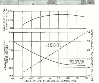
Fig. 3—Characteristics of the Y cut EDT crystal, which has its major surface perpendicular to the Y axis and its length along the X axis
