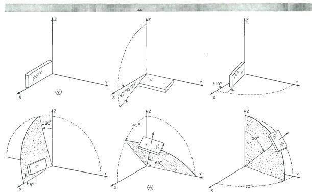
Fig. 2—There are six orientations in EDT crystals at which crystal plates with zero temperature coefficients can be cut. Two have been designated A and Y.
