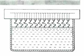
rig. 6-Method of mounting spring assemblies. If he holder is horizontal all the springs will have the ame length when pointed. In practice 40 to 100 vires are pointed simultaneously
