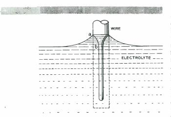
Fig. 2-Drawing of tungsten wire at one stage of the pointing action. The decreased rate of solution inside the meniscus results in the taper between a and b
