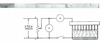
Fig. 4-Electropointing circuit. A potential difference is maintained between the tungsten wires and the cathode throughout the pointing action
