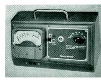
The 753-E Volume Indicator shown at the right has been developed by Bell Telephone Laboratories for maintenance work on mobile radio telephone equipment
