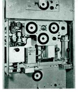
Fig. 6--Front view of stabilized microwave oscillator panel
