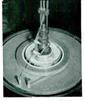
Fig. 4—Close-up of the tape insulator showing the application of the polyethylene tape over the string insulated wire
