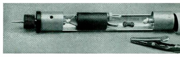
Fig. 1-The 598A tool for high impedance probing
