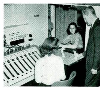
R. I. Wilkinson observing the process of starting a call in the machine on which the load carrying capacity of No. 5 exchanges is being explored. With him are left, Catherine Durnan, who handles the marker position, and Mary Tracy, who originates the calls and determines which subscriber lines are idle or busy
