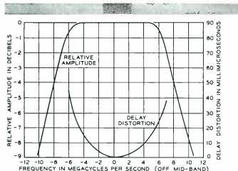
Fig. 9–Amplitude and delay distortion characteristics of a repeater of the New York-Boston system, without equalization
