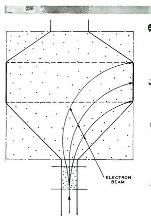
Fig. 3-Cross section of the tube in the plane of x electron beam showing schematically the bending the beam
