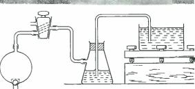
Fig. 5–Pump-siphon apparatus for variation of th level of the electrolyte. Pressure from the rubbe bulb forces liquid from the auxiliary container int the main vessel. Reversing the stopcock permit the liquid to siphon back
