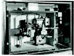
Fig. 7-Rear view of stabilized oscillator panel
