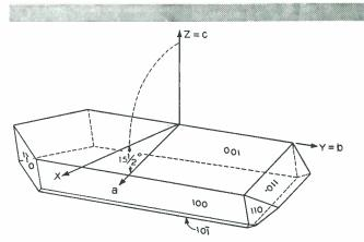
Fig. 1-EDT crystals are classified as monoclinic. They have two axis, a and c, with a 105-degree angle between them and a third axis, b, perpendicular to the others and parallel to the crystal's length
