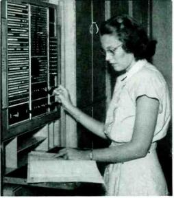
calculations. A power control panel for the computer (above left) closely resembles a type used in telephone central offices. An indicator and manual control panel analogous to trouble indicator panels in crossbar offices is shown at the right above. Facilities are here provided for analyzing problems as they progress and for inserting computing instructions on a manual basis when required.
