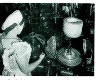
Fig. 3—An operator renews the supply on the string insulator. The insulating machine which applies the polyethylene tape is shown at the right
