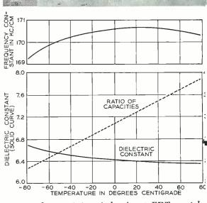
Fig. 5-Characteristics of the A cut EDT crystal. frequency variation with changes of temperature is . half that of the Y cut
