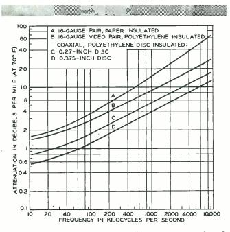
Fig. 6-Attenuation of a video pair compared with other types of circuits at video frequencies
