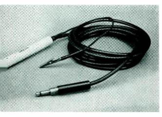
Fig. 2-The probing tool has a twelve-foot coaxial cord and plug
