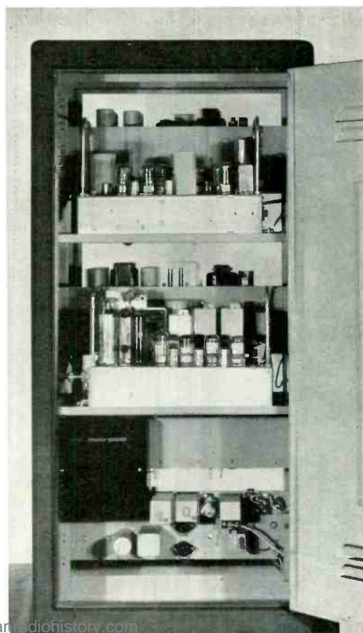
Fig. 3—Radio cabinet on subscriber's premises —power side above, radio below
