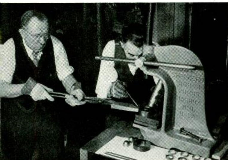
Hot Remalloy spiral segments are pressed into rings for experimental magnet production. M. Tompa holds the hot segment which D. Wallace guides to the die. In the foreground are samples illustrating the stages of processing from strip to ring
