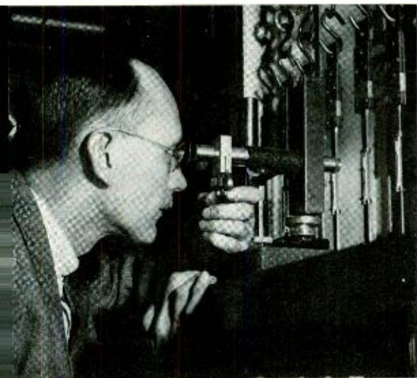
The author making a creep measurement on a section of cable sheath by means of a cathetometer which consists of a telescope moving over a graduated scale
