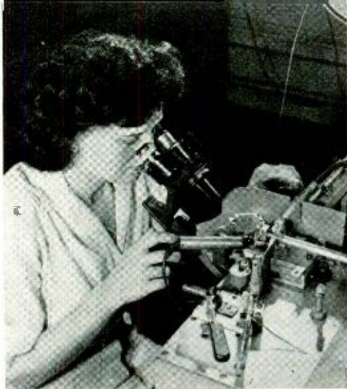
Small wires are soldered, under a microscope, at the nodal points of quartz-plate vibrators. Rose Mancuso is the operator
