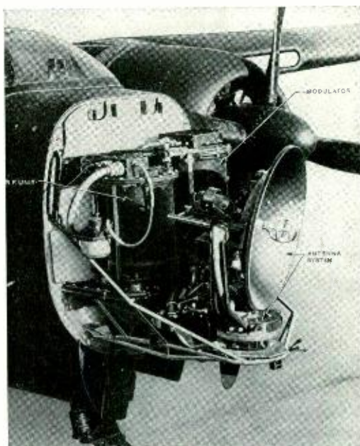
Fig. 6—The radar antenna consisting of a rotating dipole in the center of a parabolic reflector is mounted in the nose of a ship
