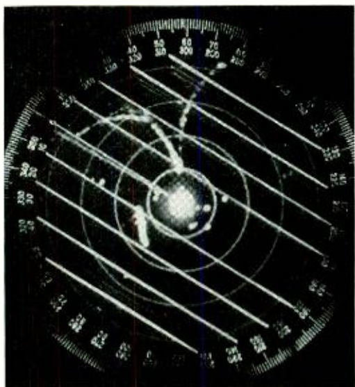
Fig. 5—A typical scope picture using five-mile range circles. North index evident at 58 degrees of the outer scale, and the ship's heading marker at 2 degrees of the inner scale
