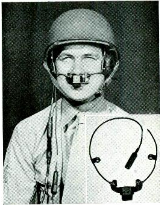
Fig. 10—The lip microphone secures quiet transmission by balancing out the noise
