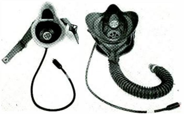
Fig. 6 (left)—A shield is used to exclude noise from the transmitter. Fig. 7 (right)—Aviator's oxygen mask also serves as a noise shield
