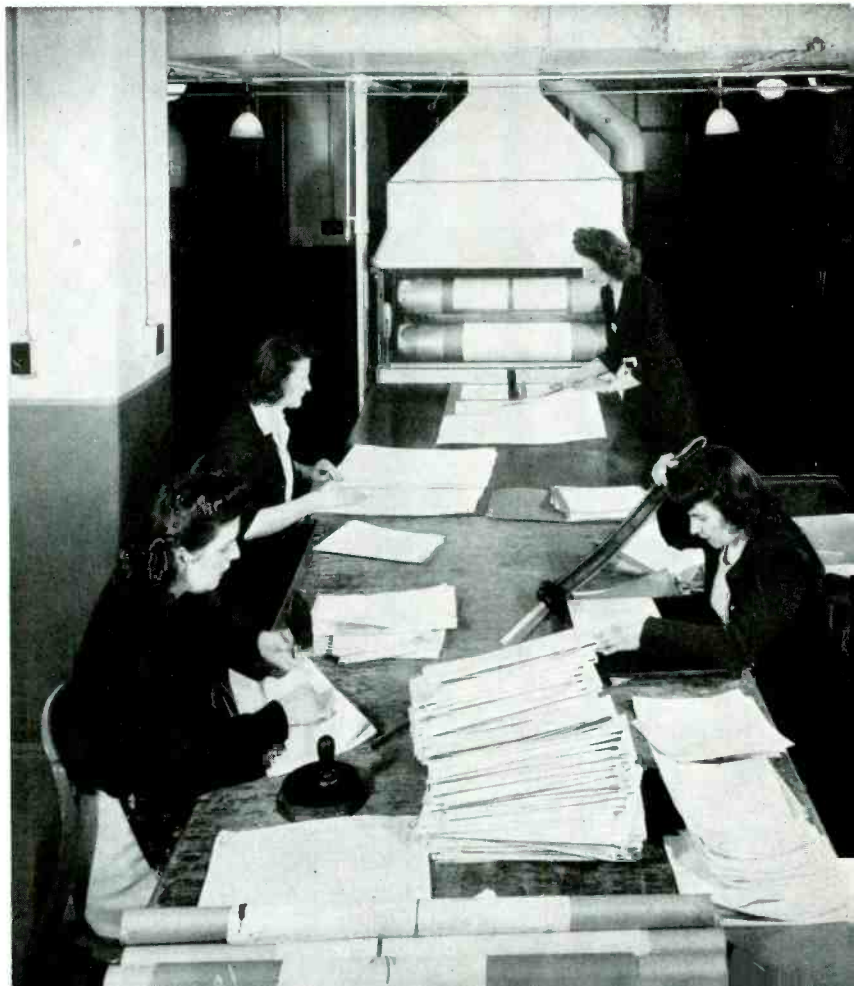
Fig. 1—Rear of a blueprint machine showing sorting, trimming, and folding team
