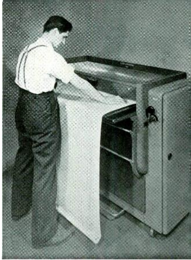
Fig. 6—The contact printer must be operated in a dark room
