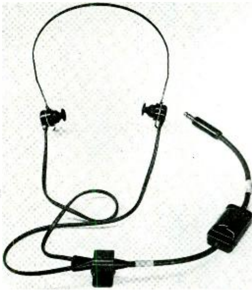
Fig. 3—Small headset receivers of the audiphone type designed for fitting under the steel helmets used by servicemen
