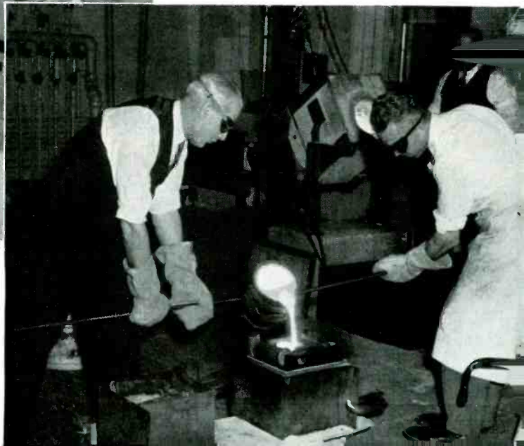
The molten metal from the furnace in the background is poured into a stack of cores. Left to right, O. J. Finch, J. M. O'Brien and O. J. Barton
