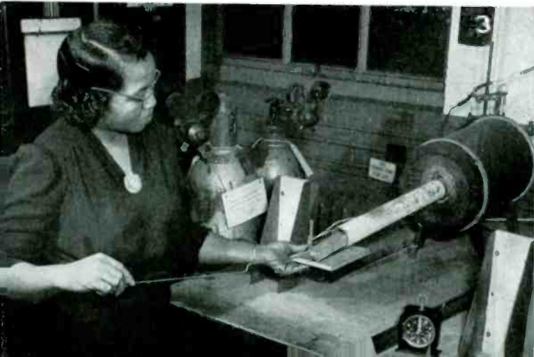
3—In this hydrogen furnace which Lillie Gibson is operating, the metal details are de-gassed and cleaned before being sealed in the glass tubing
