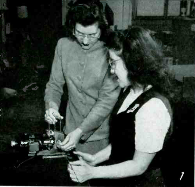
1—Helen Krisalis is demonstrating to Katherine Bliiotis the first step in making mercury contact switches, which is the wire cutting operation
