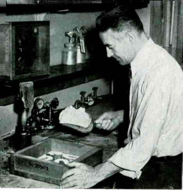
After dusting the patterns with parting sand, Mr. Wallace fills the core box
