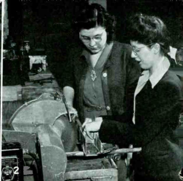
2—Marie Zvaleko watches Ann Belmont cut the glass tubing which eventually will form the envelope in which the metal details of the switch are sealed
