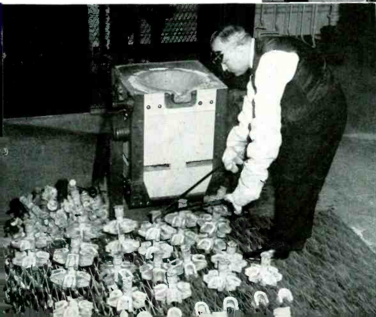
After the castings have solidified completely, they are shaken out of the molds, placed on a cooling bed, and finally separated from their gages and risers
