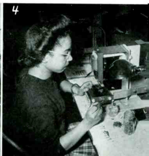
4—Here Joyce Ford is electrically welding a sub-assembly of the switch
