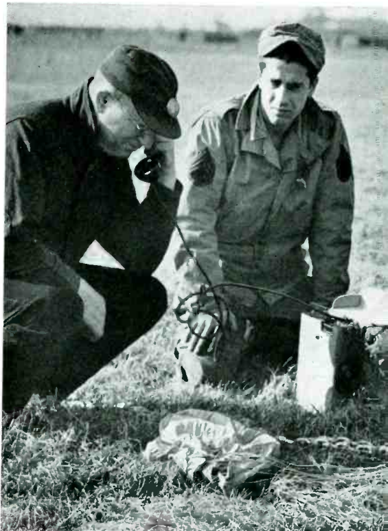
After the end of the wire is dropped to the ground by parachute and chain weight and connected to a field telephone set, conversation can be carried on over the wire between plane and ground. W. M. Bishop, shown in the plane in the above photograph, talks to H. G. Jordan, shown in the photograph at the right
