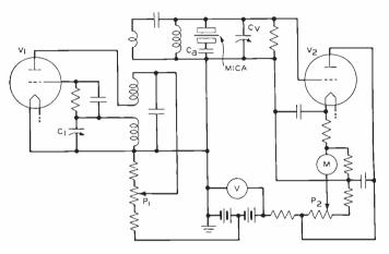
Fig. 2—Circuit schematic of the mica test set with filament supplies and power and voltage switches omitted
