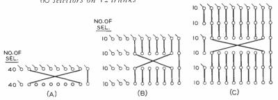
Fig. 5—Three of the graded multiple arrangements that would now be used in place of those shown in Figure 4 provide: at A, 160 selectors on 20 trunks; at B, 60 selectors on 27 trunks; NO. OF SEL.
