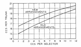
Fig. 6—Capacity per trunk for various selector loads with the old and new arrangements
