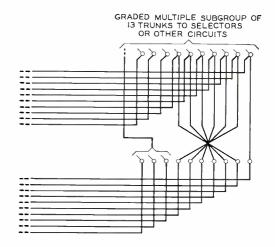
Fig. 3—With graded multiple some of the trunks are accessible to only part of the selectors. The arrangement shown forms a subgroup of thirteen trunks of which seven are accessible to all selectors
