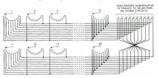
Fig. 1—With a non-graded subgroup of twenty selectors on ten trunks, all the selectors have access to all the trunks, as indicated by the cross-connections at the right
