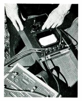
Fig. 3—The apparatus is a direct-current ohmmeter. A switch connects any one of five circuits through different parts of the pole under test. Power is supplied by three fortyfive-volt dry batteries in series
