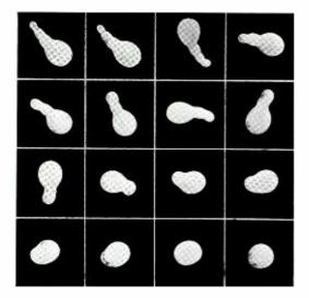
Fig. 3—Progressive stages in the merging of Hevea particles. Two or more small particles become attached to a large spherical one. They are slowly absorbed and form a larger sphere
