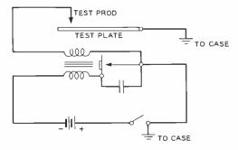
Fig. 4-Circuit schematic of the spark test set
