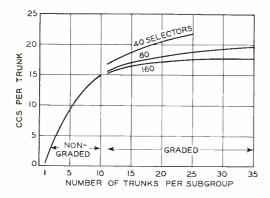
Fig. 2—The capacity in CCS per trunk for non-graded trunk subgroups from one to ten and graded subgroups of eleven to thirty-five trunks based on 1/100 lost calls
