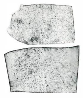
Fig. 7—Both of the above sheets of spotted and stained mica would be rejected by visual inspection, but the mica tester shows the sheet at the top to be of electrical quality F.3, while that at the bottom is F.1
