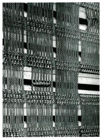
Fig. 7—Close-up of DTA frame showing a twelve-trunk graded group near the center
