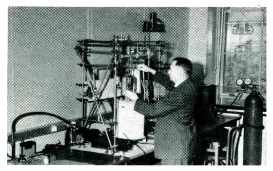
Pumping apparatus used in studying the physical properties of thin films. H. G. Wehe is carrying on the investigation
