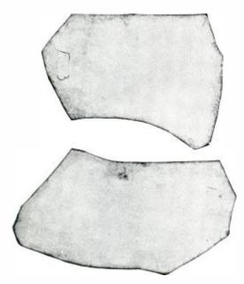
Fig. 6—Both of the above sheets of ruby mica would be accepted by visual inspection, but a reading on the new mica tester would show the sheet at the top to be of electrical quality E3, while that at the bottom is Ex
