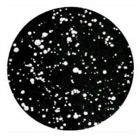
Fig. 1—Balata latex, enlarged from one frame of a motion picture of the particles. The small particles rotate around the larger ones
