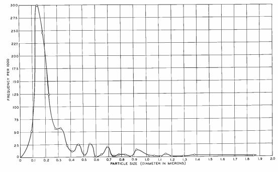
Fig. 5—Most of the particles of Hevea latex are less than 0.30 microns in diameter but those which are larger contribute most to the total mass
