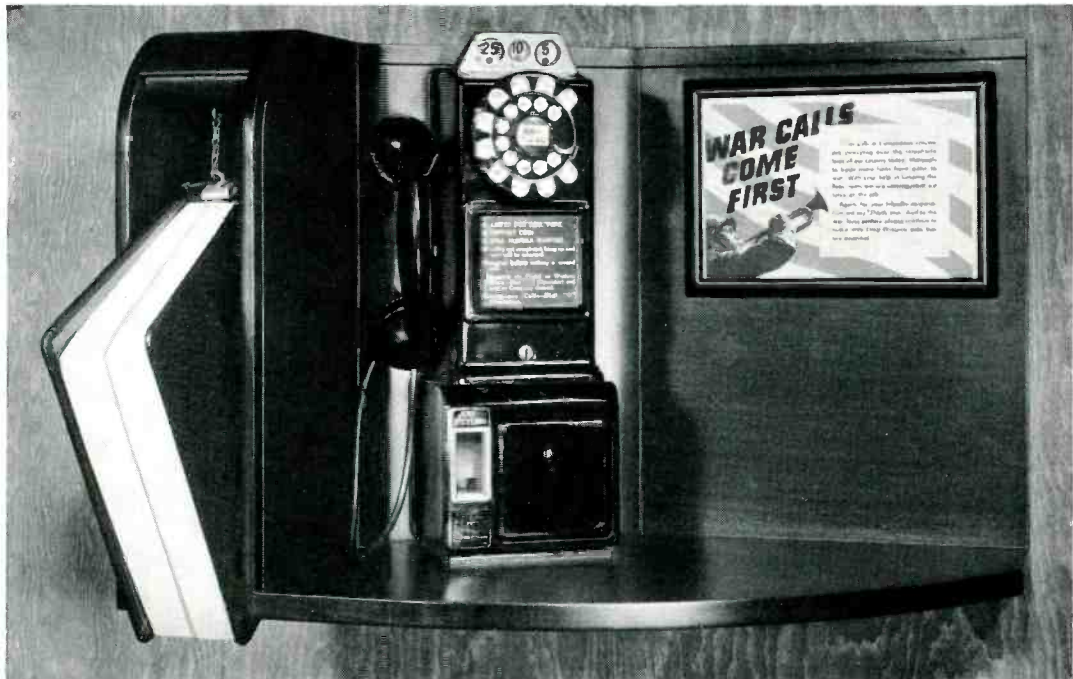
Besides a coin collector, the mounting supports a suspended directory and a broad shelf for note taking and placing hand bags or small parcels
