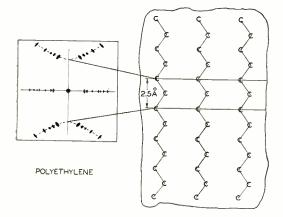
Fig. 2—Chain structure of the polyethylene molecule showing the location of the atoms which produce its X-ray pattern
