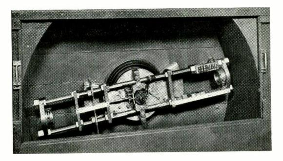
N ITS more usual form, a centrifuge is employed to separate materials of different specific gravities by the action of centrifugal force. At high rotational speeds, objects tend to be driven radially outward with an acceleration proportional to the square of velocity. Heavy particles in a rotated liquid, for example, may be separated from the liquid by this action, or on a mixture of liquids, the heavier may be separated from the lighter. The actual ac-
