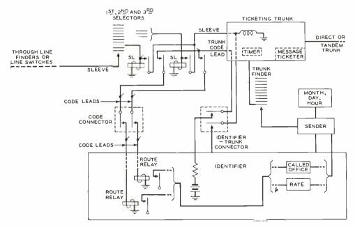
Fig. 2—Essential elements of circuit used in the automatic ticketing system to determine the called-office code dialed by the subscriber
