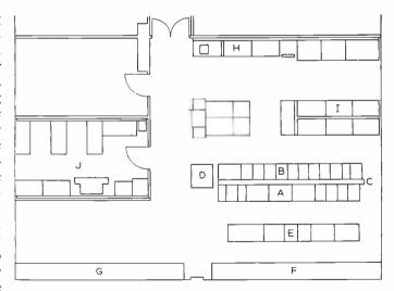
Fig. 3—Plan of the electroplating laboratory at Murray Hill. The main plating baths, A to E, are located in parallel rows near the center of the room. Continuous plating on wire is done at F; dyeing and sealing at G. The experimental work is largely carried out on benches at H and I; samples are prepared in a separate room, J
