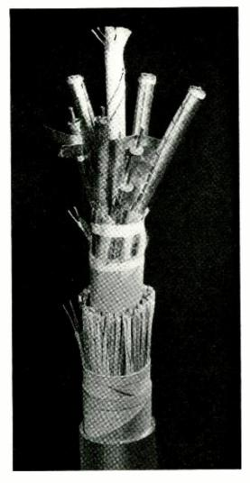
Coaxial cable now being installed between Terre Haute and St. Louis. It consists of 6 coaxial conductors, 21 quads and several service pairs
