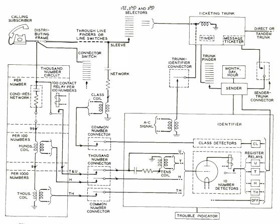
Fig. 1-Identifier circuit for the automatic ticketing system in Culver City, California
