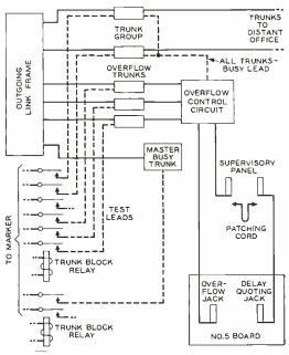
Fig. 1—Simplified schematic of connections to overflow circuit
