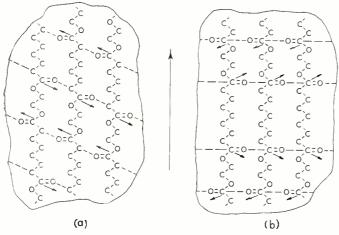
Fig. 4—Schematic of polyethylene suberate (a) and polyethylene azelate (b) molecules. The former has an even number of atoms between the C=O groups which permits stronger association with adjacent molecular layers and is therefore the stronger plastic
