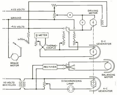
Fig. 1—Simplified circuit diagram for the 1,000-g centrifuge December 1944
