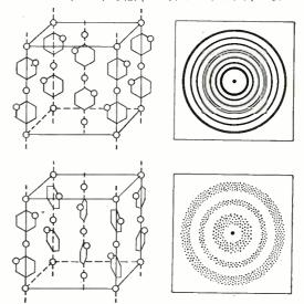
Fig. 5—Ordered (upper) and disordered (lower) cellulose chain molecules with the X-ray diagram of each. Sharp lines are obtained with an ordered specimen
