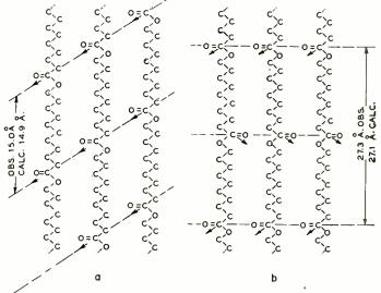
Fig. 3—Schematic of polyundecanoate (a) and polydecanoate (b) molecules showing the difference in frequency of occurrence and position of the active C=O groups which determine the strength of attraction between adjacent molecular layers and hence the strength of the plastic
