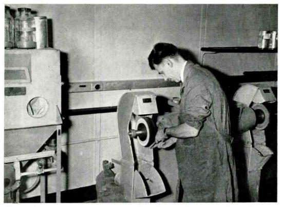
Fig. 2—The preparation room is equipped with a polishing lathe and sand-blast machine; also a bench lathe, drill press and a spot welder. G. Bittrich is shown polishing a sample
