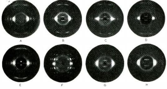
Fig. 1—X-ray patterns of synthetic plastics showing the effect of progressive changes of chemical composition and of heat treatment
